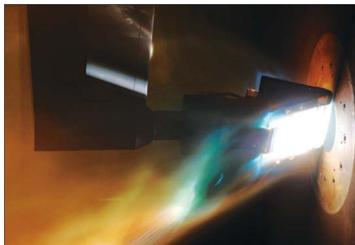
An Orion heat shield material sample model undergoes aerothermal testing in H2 as part of a recent facility validation and calibration run. This and other heat shield material candidates will undergo aerothermal pre-production testing at AEDC in June.
