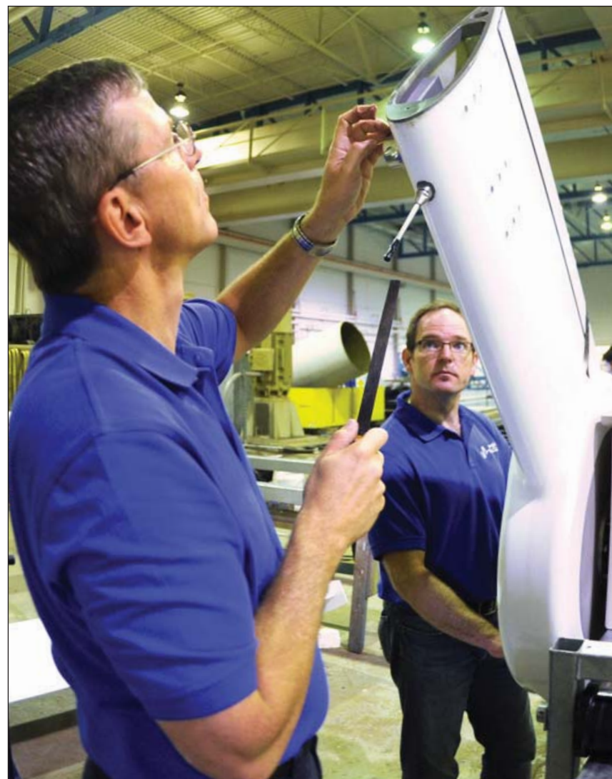
Retired Col. Rob Fredell files a metal socket on the pylon, which will connect the blades of the wave energy converter
