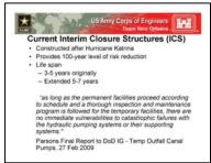
The ICS's were constructed after hurricane Katrina and currently provide 100-year level of risk reduction. In the beginning, their life span was three to five years because we were hoping to get a permanent pump station within three to fiver years. We have done some maintenance work on the structures which would allow the ICS's life span to extent to five to seven years. An independent evaluation performed by Parson's Engineering found that as long
