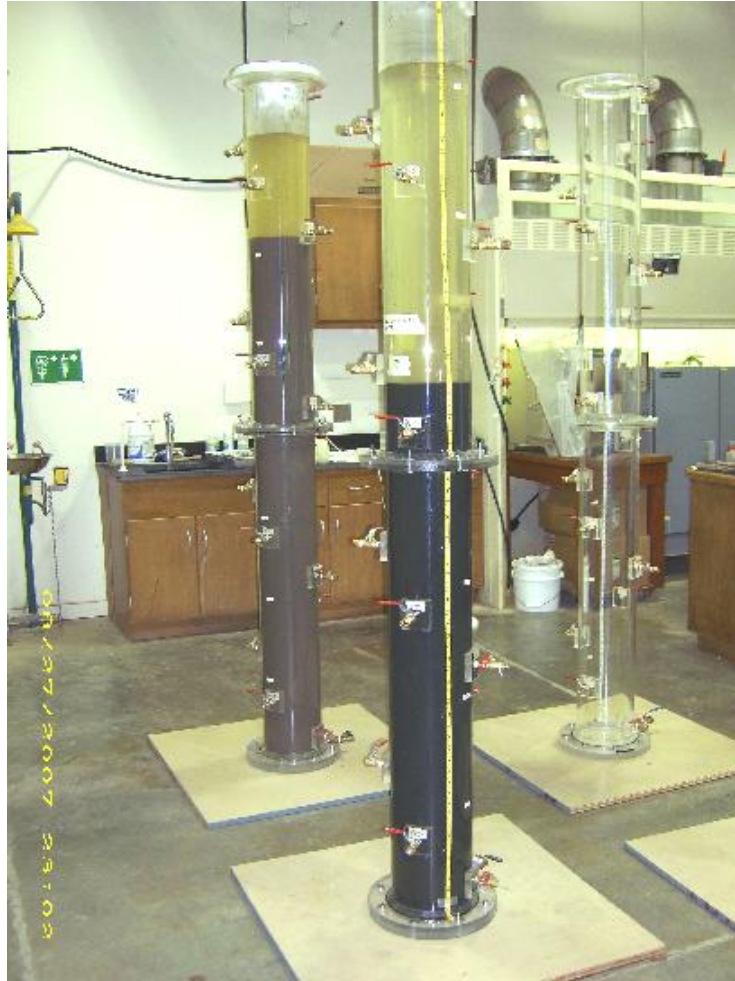
Figure 8. Column Settling Test
