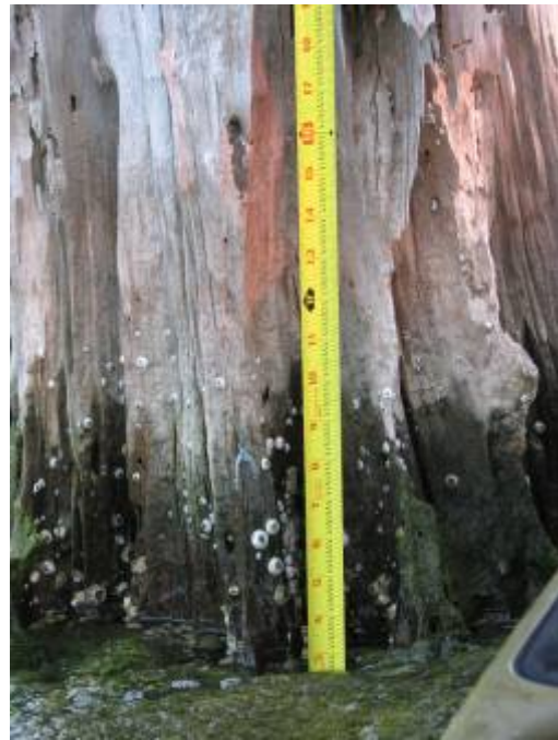
Figure 28. Tidal range measurements taken at wall (left) and stump (right) in area near proposed mitigation site.
