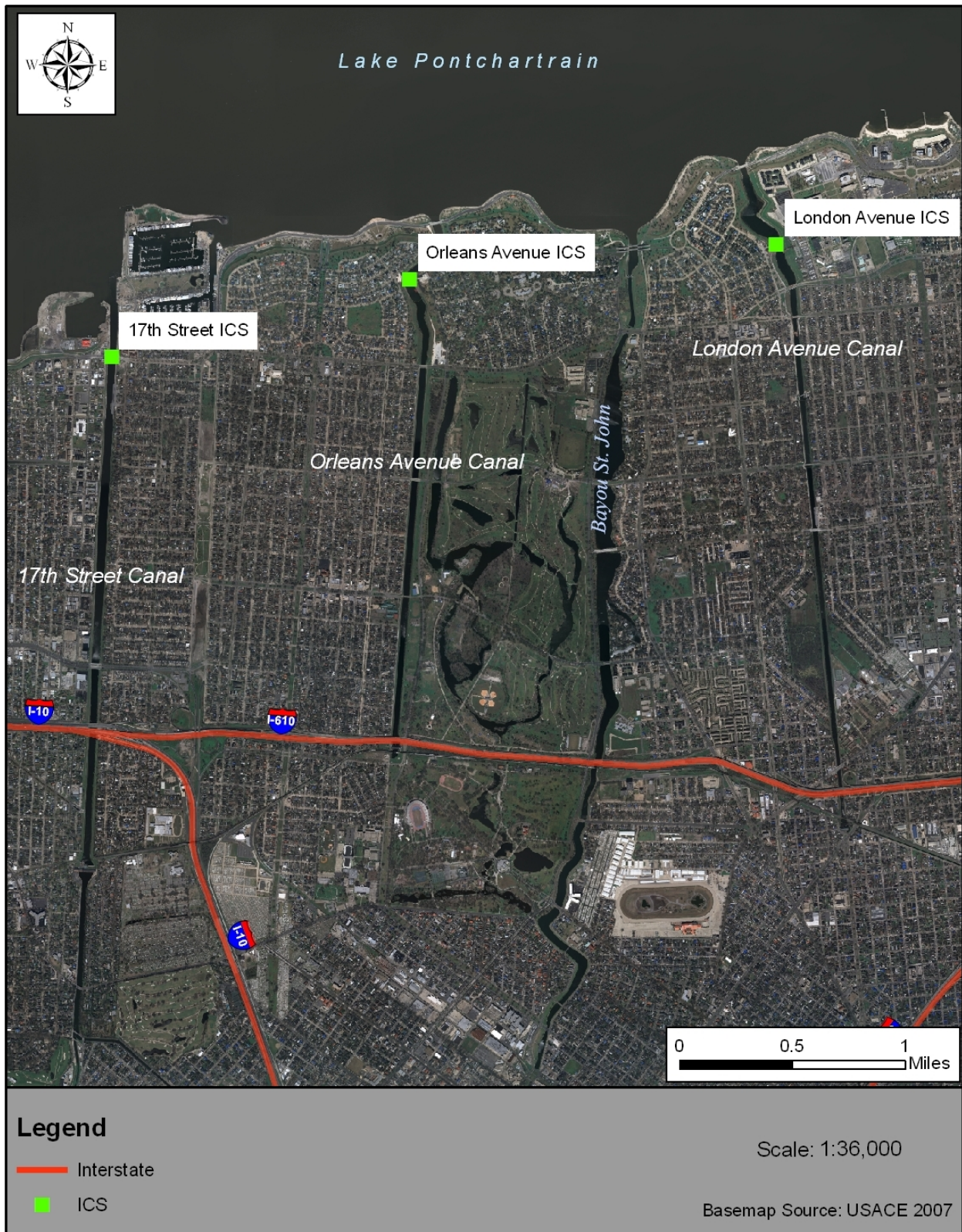
Figure 16. Locations of Interim Closure Structures
