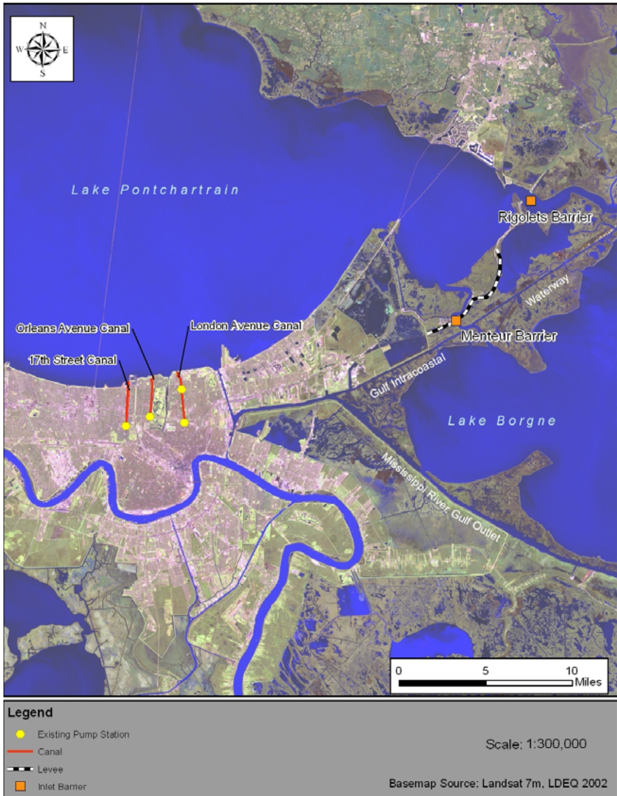
Figure 18. Lake Pontchartrain Barrier Plan
