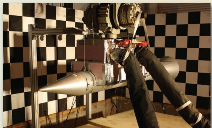
B61-11 instrumented test unit and temperature-conditioned ejection rack.
