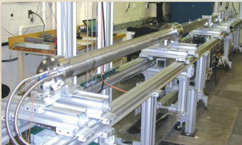
The left photograph shows the multiphase shock tube that uses a dense particle curtain (right top) impacted by a shock wave (right bottom) to produce shock-particle interactions.
