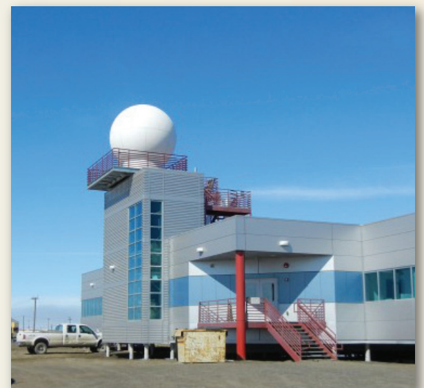
A newly installed X-band scanning ARM precipitation radar operates from atop the Barrow Arctic Research Center.
