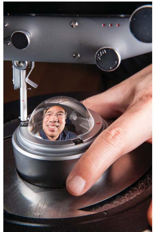
REALLY ROUND — The image of project lead Hy Tran (2541) is reflected in a polished quartz ball that is the standard for roundness. The Primary Standards Laboratory at Sandia uses a specialized instrument to measure roundness deviation against the roundness standard, which has been certified to national standards to be round within about 20 nanometers. (Photo by Randy Montoya)
