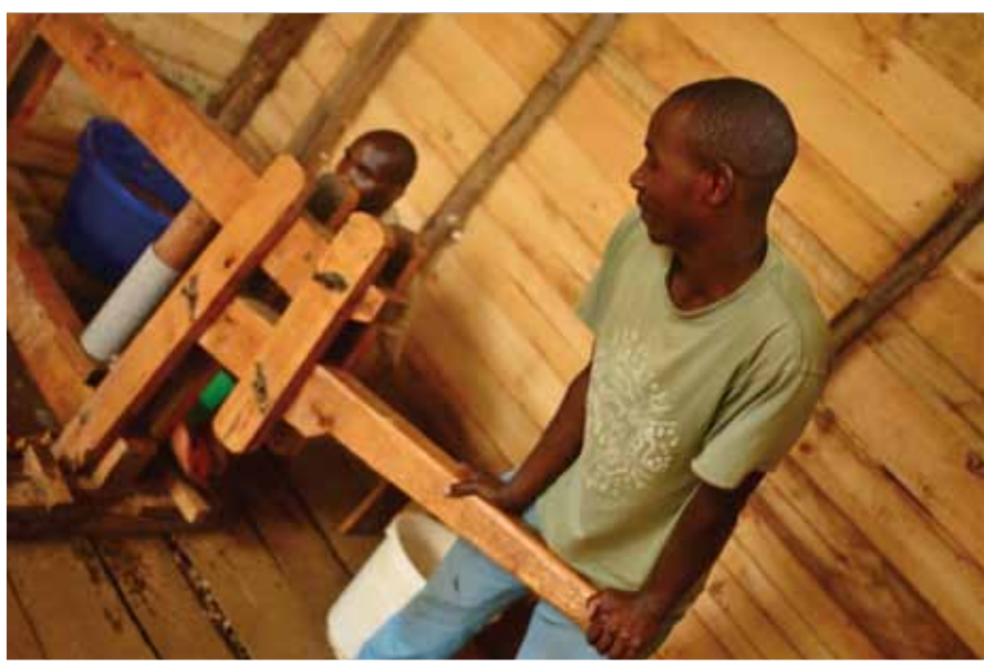
A member of Volunteers Jarod and Sarah Ring's community uses a press to make briquettes. Used as an alternative to charcoal, the briquettes are made from sawdust left over from local carpenters and scrap paper from the local schools.
