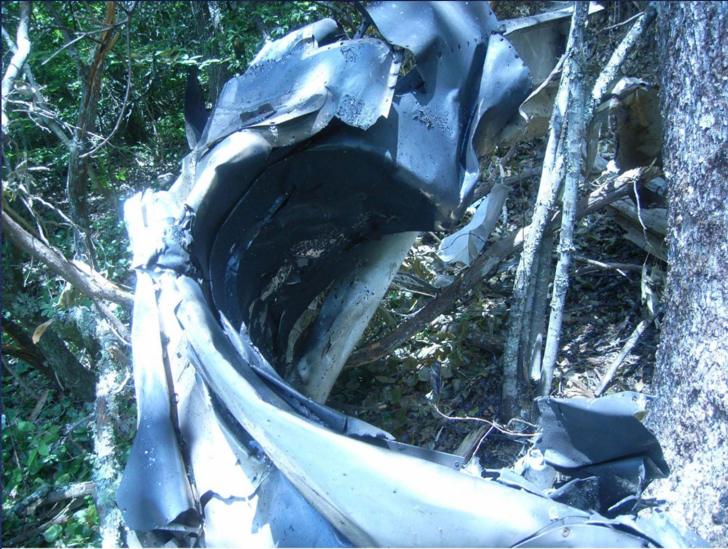
Photo 3 - Left Wing, concave depression
