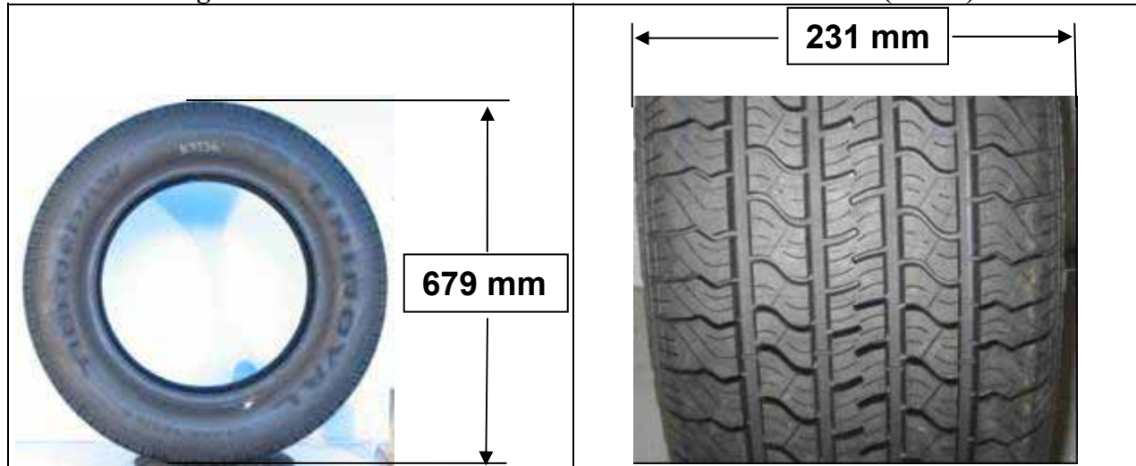
Figure 11. ASTM F2493-06 Standard Reference Test Tire (SRTT)
