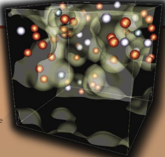
Quantum molecular dynamics simulation showing the atomic nuclei and an electron density iso-surface for stainless steel at high energy density. These simulations are being used to calculate the electrical and thermodynamic properties of stainless steel and other materials under the extreme current densities found on the Z machine.
