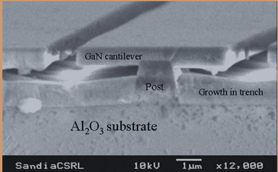
A scanning electron microscope image shows a cantilever epitaxy growth on top of the sapphire post. This Sandia-developed process for growing gallium nitride on an etched sapphire substrate may help light up the world with brighter green, blue, and even white high-efficiency light-emitting diodes.
