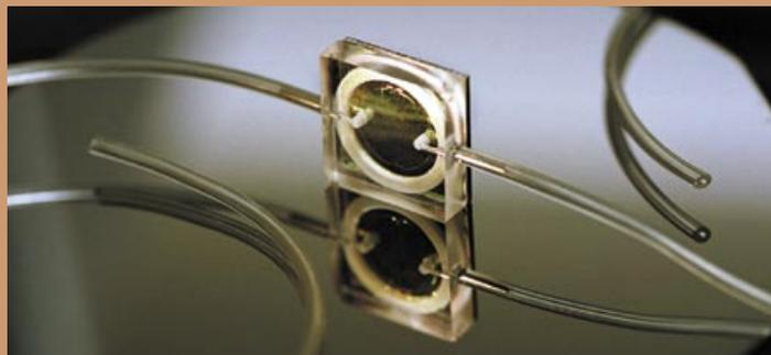
The BioCavity laser is based upon the Vertical Cavity Surface Emitting Laser, a Sandia-developed technology. A completed device with tubing to allow the flow-through of samples is shown here.
