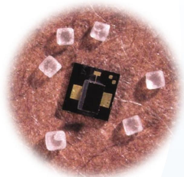
Verifying the desired atmosphere inside hermetic devices becomes much more difficult as package size decreases. Sandia researchers have developed methods and hardware to successfully sample and analyze the internal gas atmosphere of nanoliter packages (shown here with salt gains).
