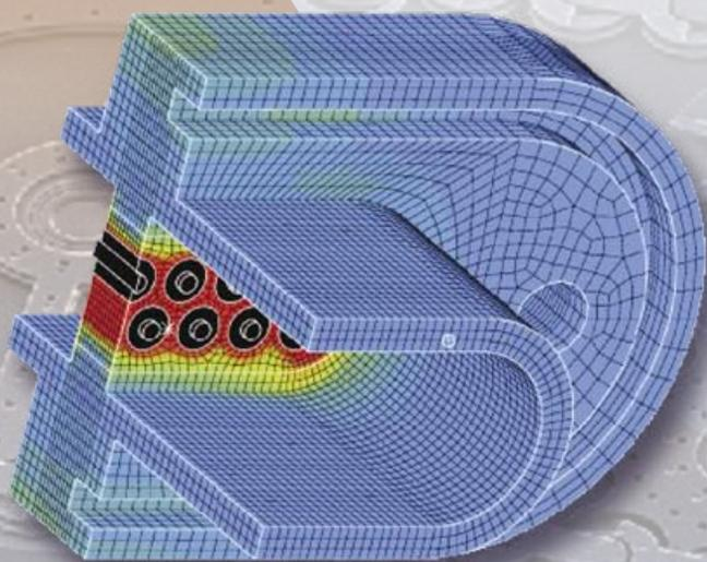
This high-fidelity simulation of a 15-pin hermetic microminiature connector shows the stress generated in the housing by glassing operations. Simulations, like this one, support changes in manufacturing processes to improve product yield. This two-minute simulation took about 24 hours to do a decade ago.
