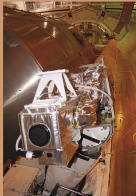
Sandia's orbiter inspection sensor housed in the payload bay (above) and being used to reach out toward the shuttle wing to scan tiles (left).
