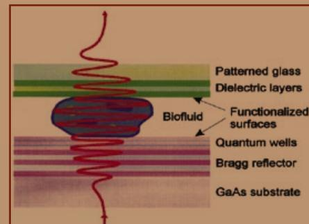
The laser cavity is fabricated with a space (a microfluidic channel) to allow the passage of whole cells or other biological material, as illustrated here.
