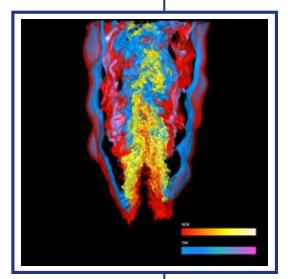
Jacqueline Chen employs some of the world's fastest supercomputers to gain insight into the flames that ignite and stabilize diesel-engine jets. Photo courtesy Sandia National Laboratories.
