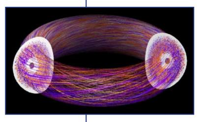
Small eddies created by plasma turbulence are shown in cross-section along with the magnetic field lines threading the simulated tokamak.
