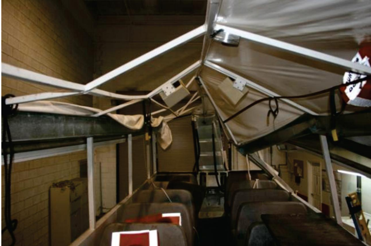
Figure 7. View of DUKW 34 's damaged canopy, looking aft.
