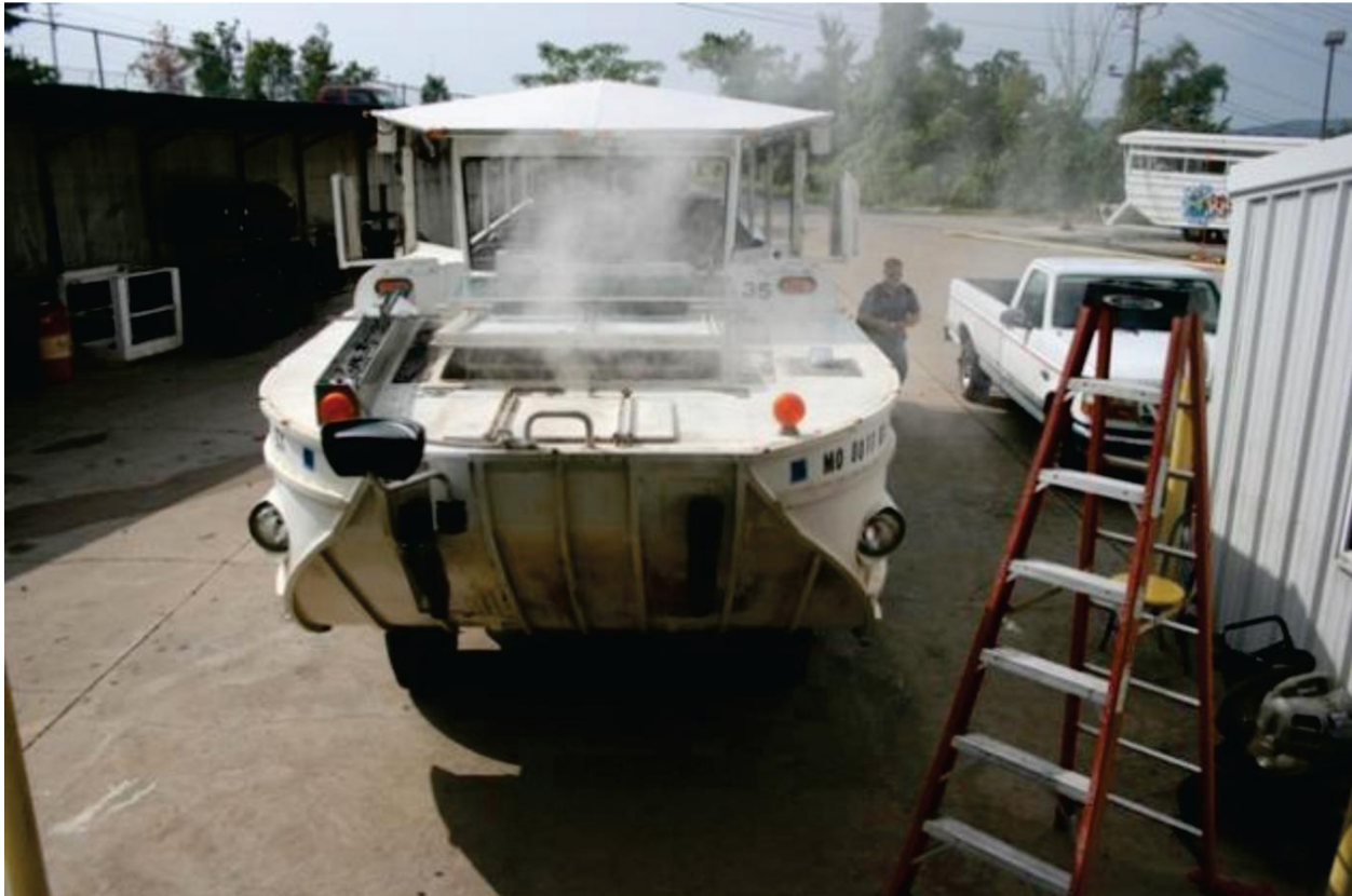
Figure 10. Steam from the engine compartment of a test APV, with cooling water temperature of about 220° F.
