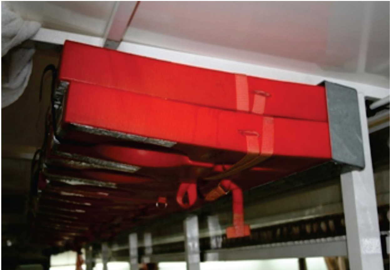
Figure 8. Lifejackets on Ride the Ducks APVs were stowed in stacks of two above each row of passenger seats. Adult jackets were on the starboard side; child jackets were on the port side.
