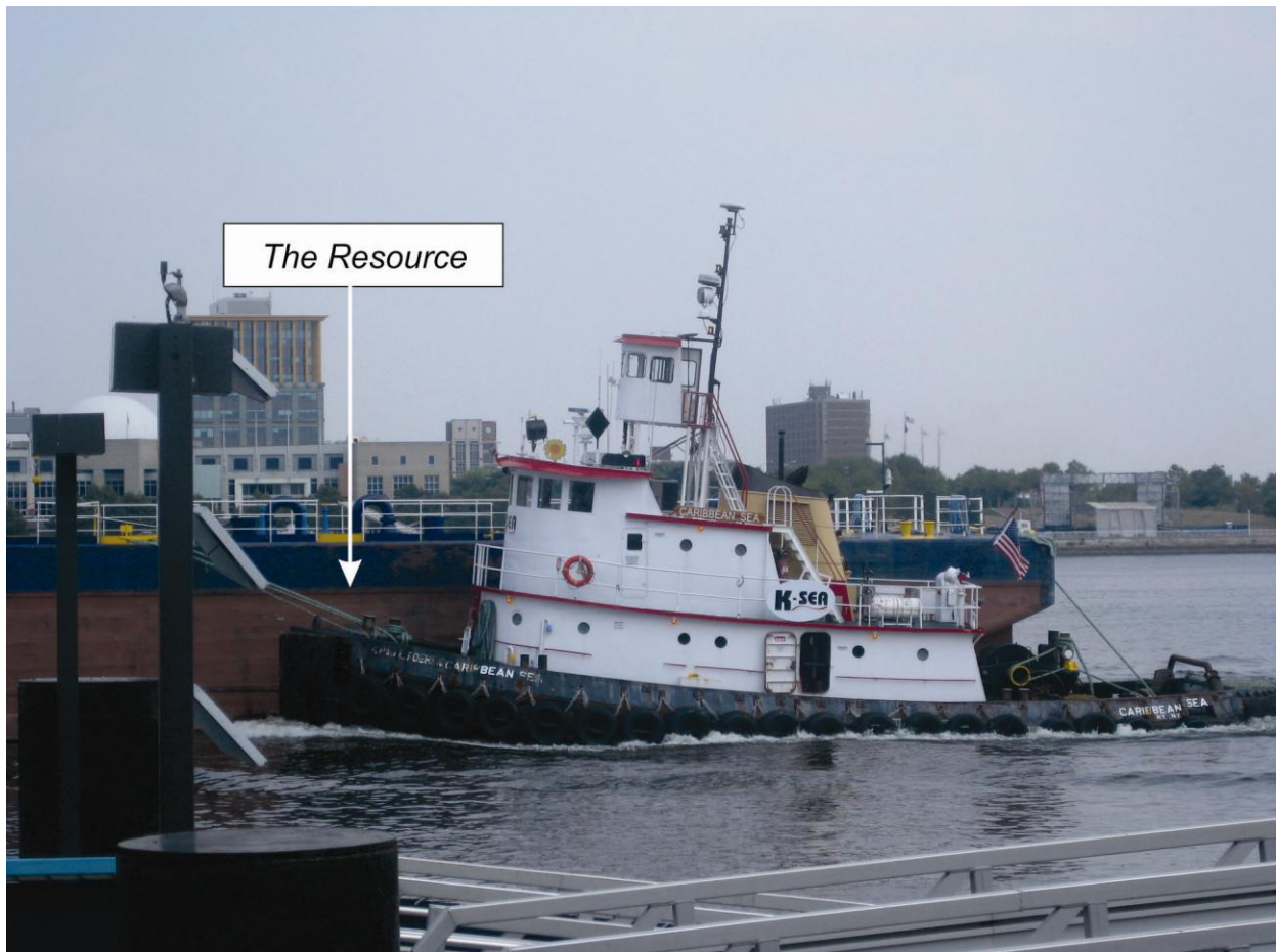
Figure 3. Tugboat Caribbean Sea with tank barge The Resource in a starboard hip tow as seen about 45 seconds before the accident. (Photo by Megan Scharpf)
