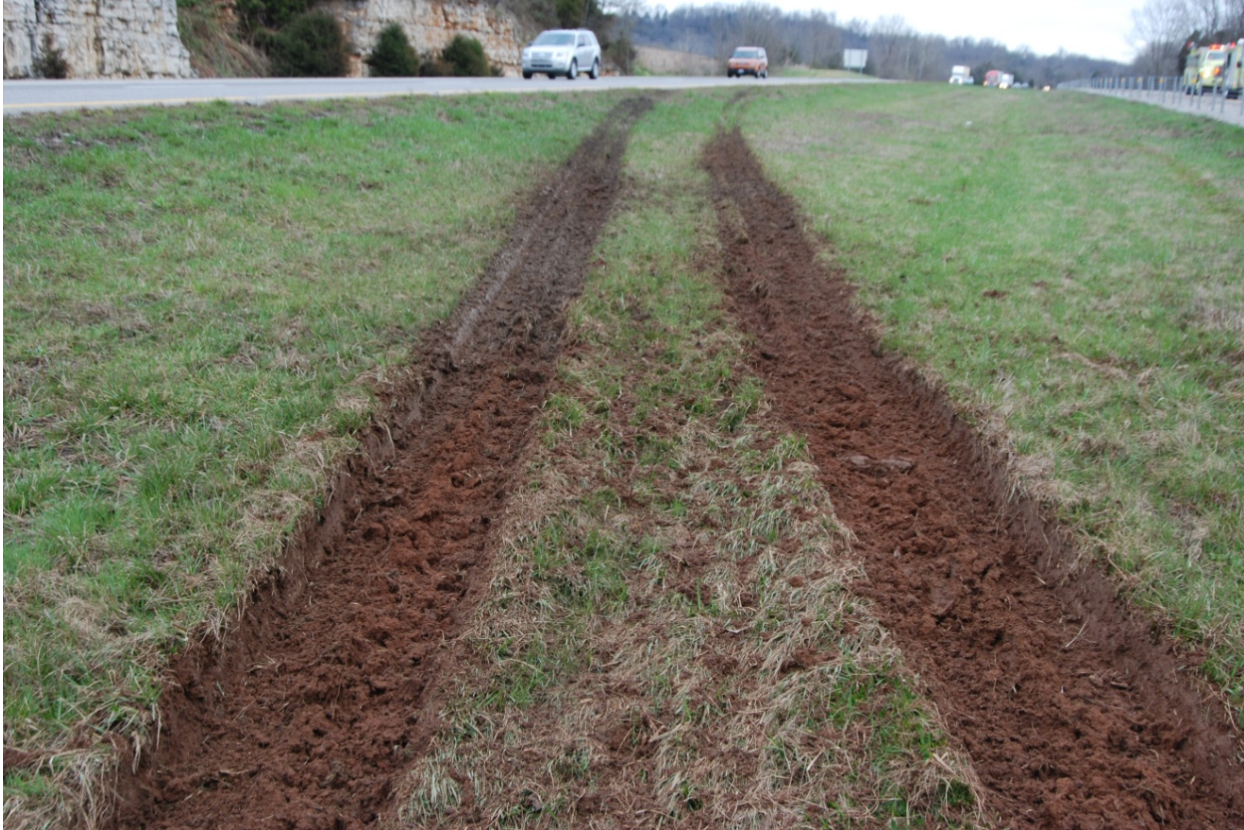
Figure 9. View looking north of truck tracks across the median, showing furrows from brake application.
