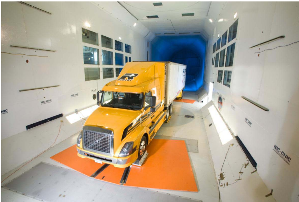
Figure 3-4: Full-scale, fixed floor test in the NRC 9-meter wind tunnel (model tested for this program not shown).
