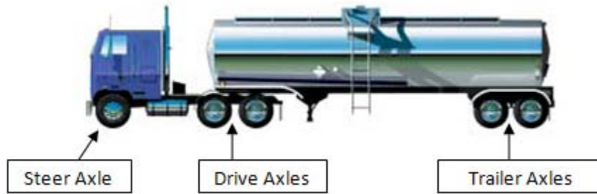
Figure 1-19 Class 8 Standard "18 Wheeler" Axle Identification
