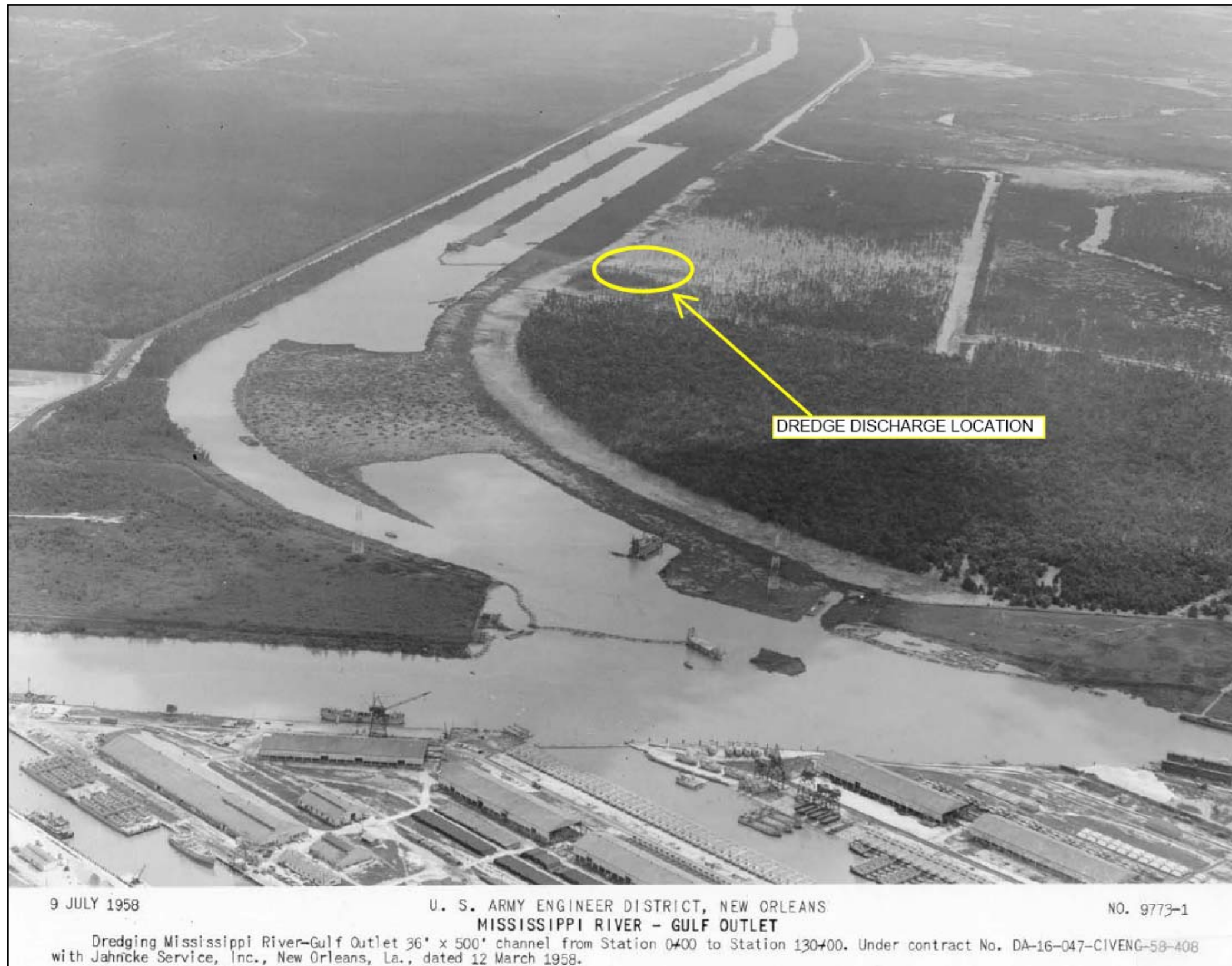
Figure 6. Historical photo - discharge to the MRGO disposal site during dredging of the Mississippi River Gulf Outlet 1958.
