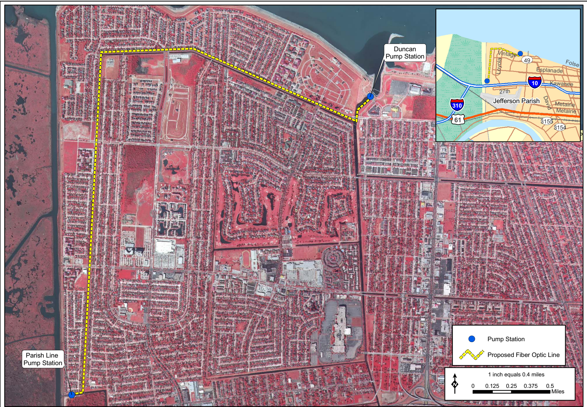
Figure 4a: Fiber Optic Line From Parish Line Pump Station to Duncan Pump Station
