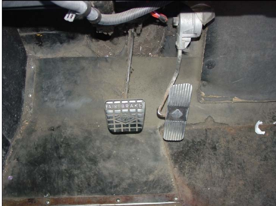
Figure 6. Pedal configuration of Nanuet accident bus (Bluebird), with accelerator and brake pedals on same plane.
