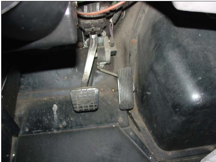
Figure 7. Pedal configuration of Nanuet driver's usual bus, showing accelerator set farther back than brake pedal and accelerator mounting below accelerator pedal.
