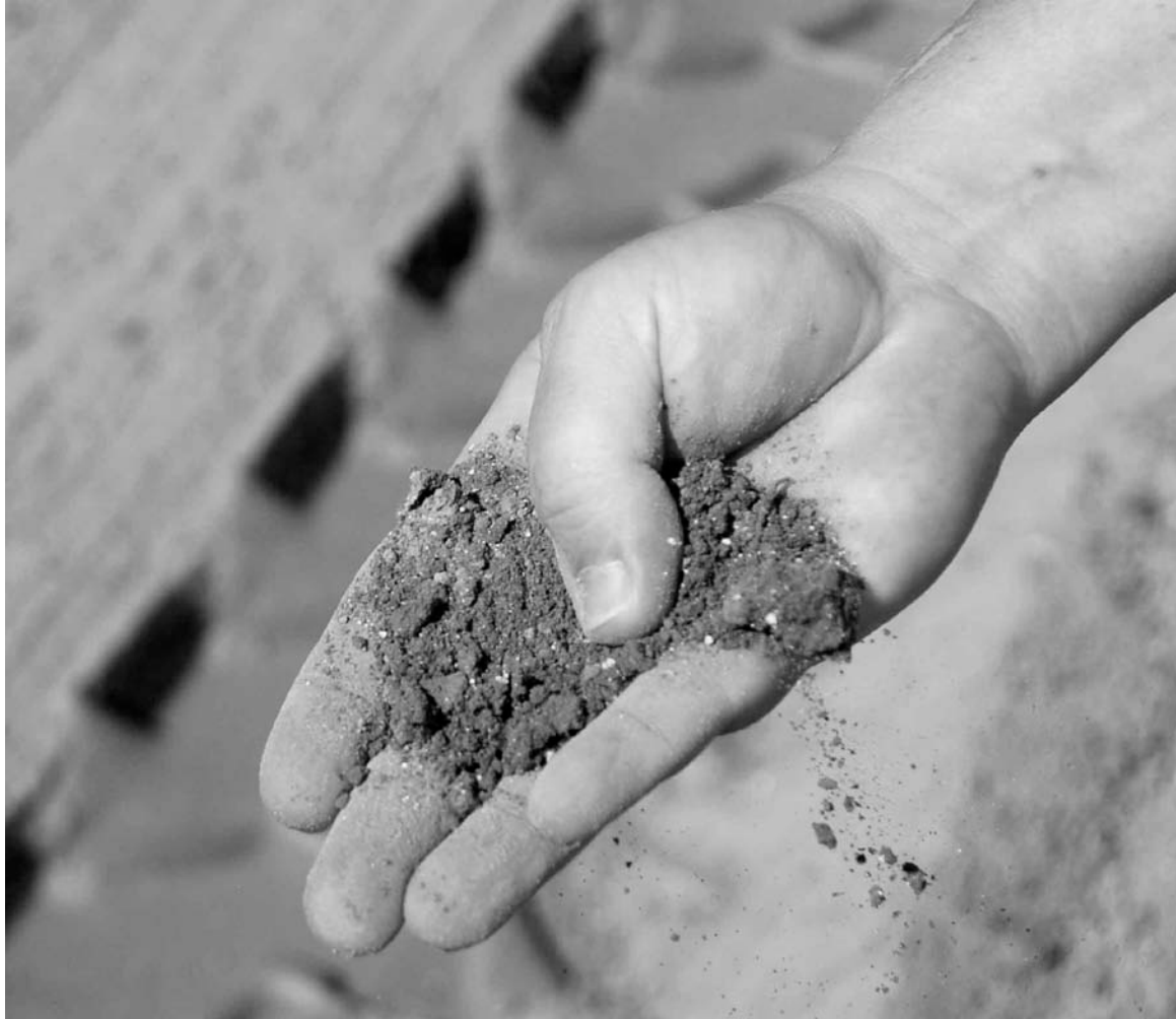
Figure 17. Lime and Soil Mixture
