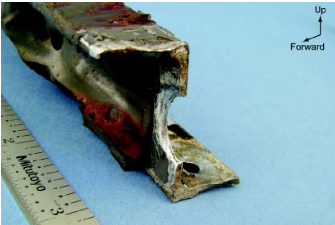
Figure 5. Right Wing Rear Z-Stringer Fracture
