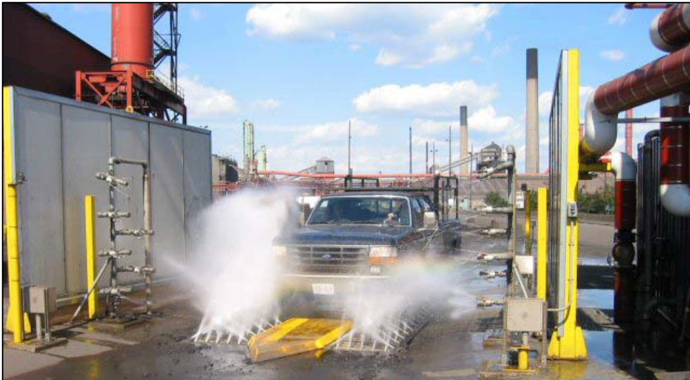
Figure B-5. InterClean Equipment's heavy duty washing system (InterClean, 2008).
