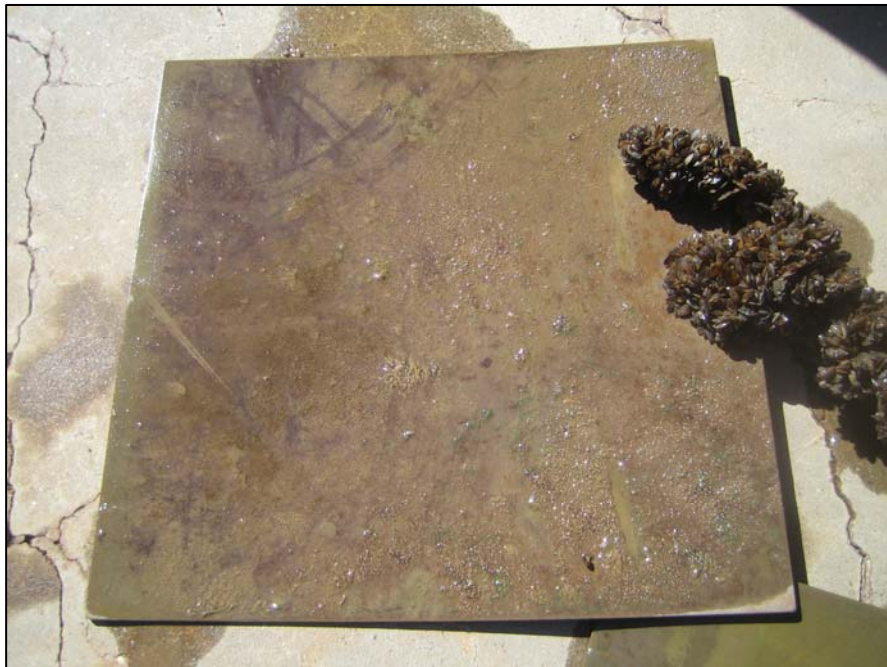
Figure B-11. This bronze plate has been submerged for 18 months in Lake Havasu; notice the rope has mussels attached while the plate is mussel free (photo courtesy of Allen Skaja, 2009).
