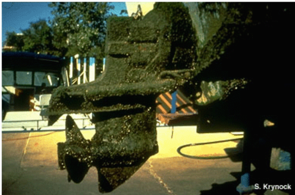
Figure A-6. Mussels on the lower unit of an inboard/outboard engine.
