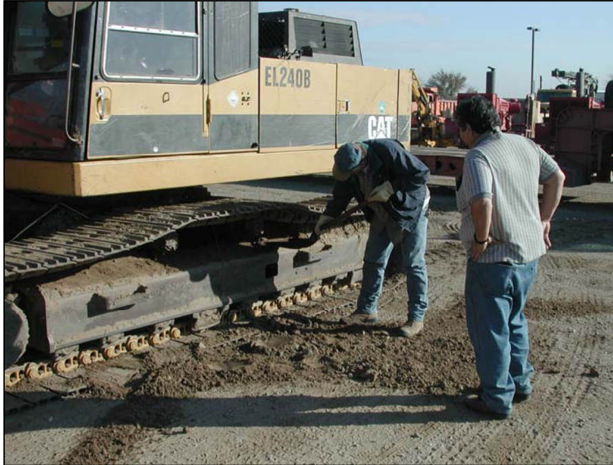
Figure 7. Precleaning heavy accumulations can help reduce water use when washing (photo courtesy of Fred Nibling).
