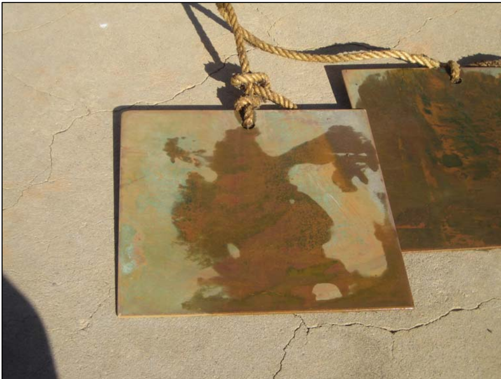
Figure B-9. This copper plate has been submerged for 18 months in Lake Havasu, notice there are no mussels on the rope or on the plate (photo courtesy of Allen Skaja, 2009).
