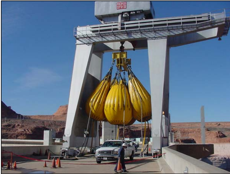
Figure 11. Crane testing at Glen Canyon Dam (photo by Gerry Jarin; photo courtesy of Jim Jota, Imes, Inc., 2005).
