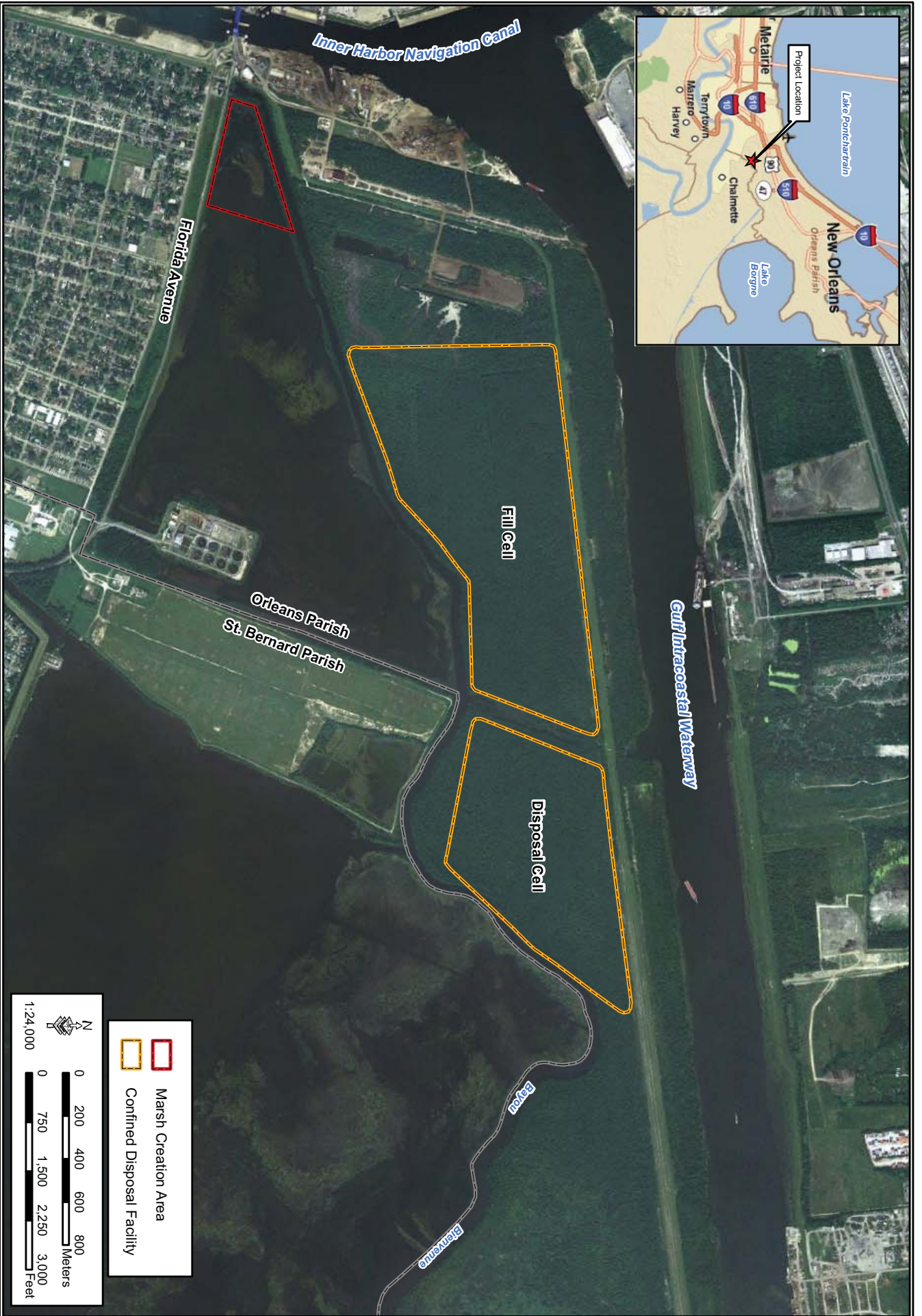
Figure 4-7: Cast-in-Place Confined Disposal Facility Option #1
