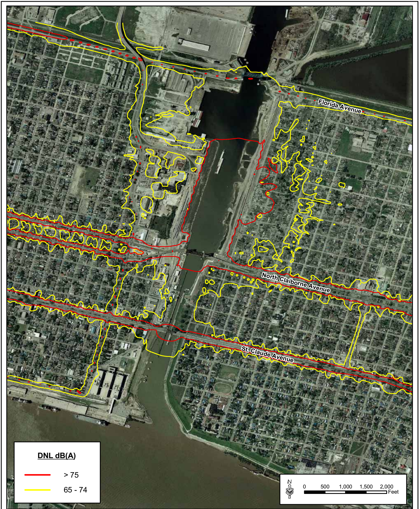
Figure 5-8: DNL Noise Contours Due to IHNC Construction, Installation of Temporary Bridge at St. Claude Avenue, and 2014 Traffic Post North Claiborne Avenue Bridge Replacement
