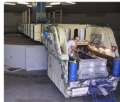
Geotechnical centrifuges with in-flight shakers, such as the 9-meter radius unit at UC Davis, play a role in understanding and quantifying liquefaction effects.
