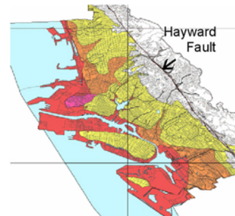
Regional liquefaction hazard map showing the California communities between Berkeley and Oakland for a 7.1 magnitude earthquake. Blue areas represent water. 73% of the red area is predicted to show surface manifestations of liquefaction, (Holzer, et al., 2002).
