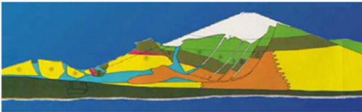
The flow failure of the upstream slope of the Lower San Fernando Dam in 1971 nearly caused overtopping, which could have killed thousands. It has been reconstructed and analyzed by Seed, et al. (1975) to provide an understanding of the mechanics of flow failures and to develop engineering procedures to evaluate post-liquefaction soil shear strength.
