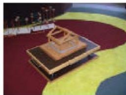
Hand-operated shake table and collapsible/re-erectable structure model, Riverside County Youth Museum
