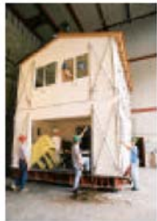
Full-scale shake table testing of a two-story house (left, UC San Diego) and three-story apartment building (center, UC Berkeley). A new engineering analysis method and software package were produced (right).
