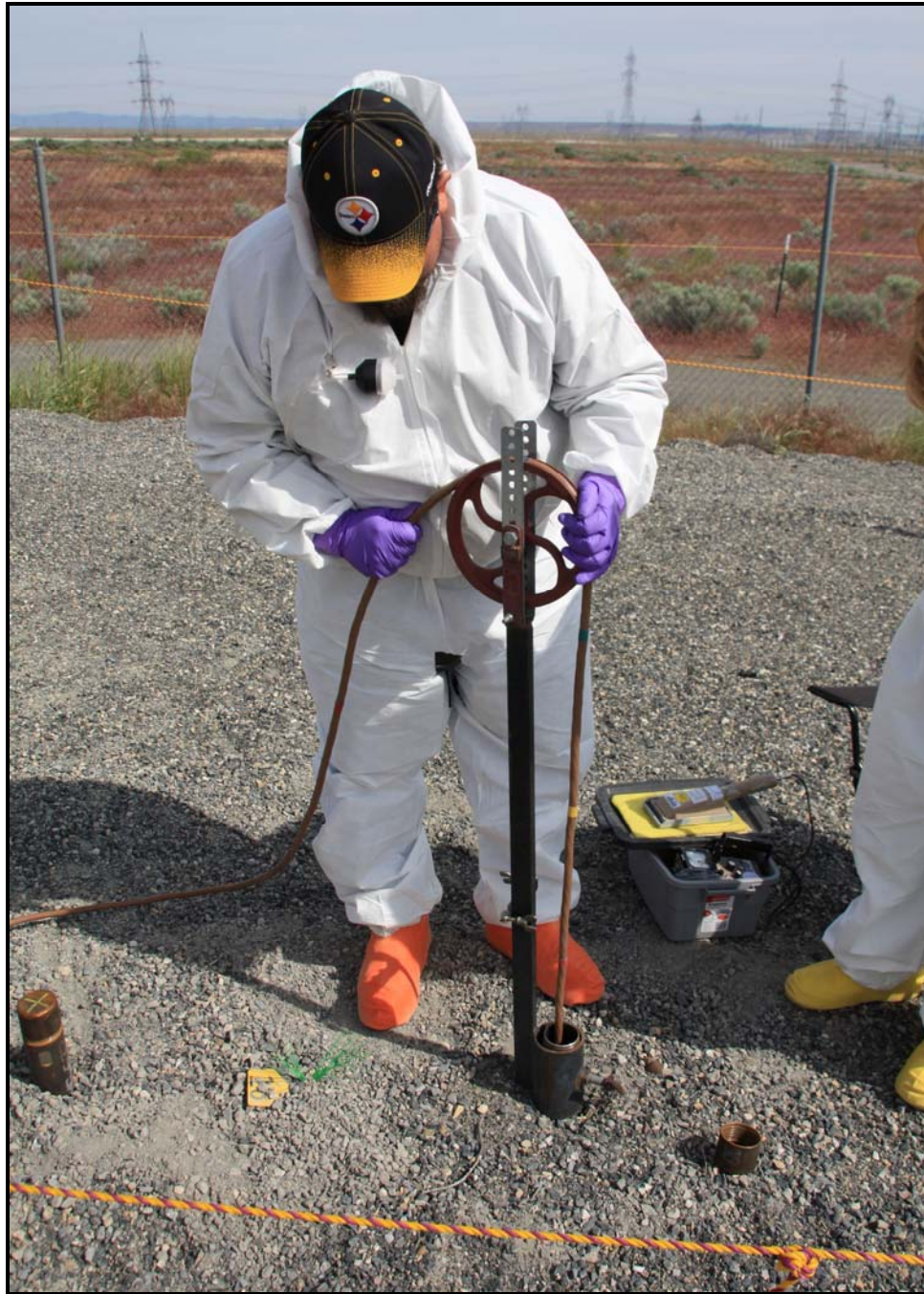
During nonintrusive characterization at the 618-11 Burial Ground, a multi-detector probe was used to identify the location of radioactive materials within the vertical pipe units. (Photo 5)
