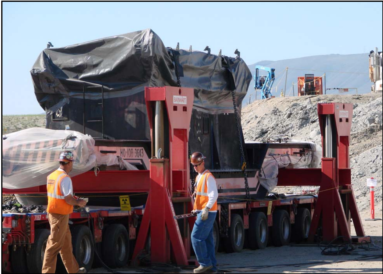
The Environmental Restoration Disposal Facility has received 7 of 11 railcars from the 212-R rail spur. The remaining railcars are expected to be delivered next week. The railcars contained lead-lined casks used to transport irradiated fuel. (Photo 2)
