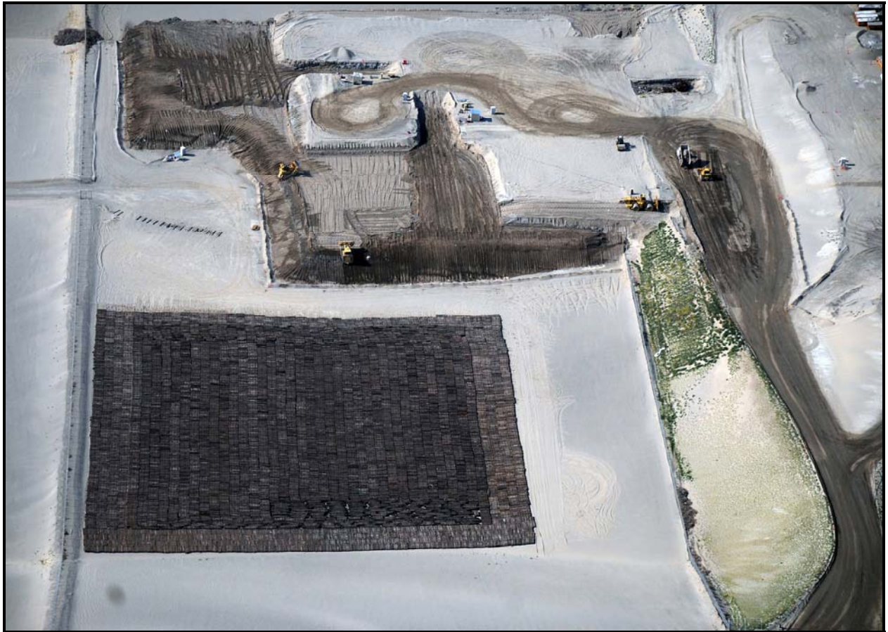
An aerial photo taken in late June shows the 58,500 Hanford Site railroad ties that were disposed in super cell 9 at the Environmental Restoration Disposal Facility. (Photo 1)
