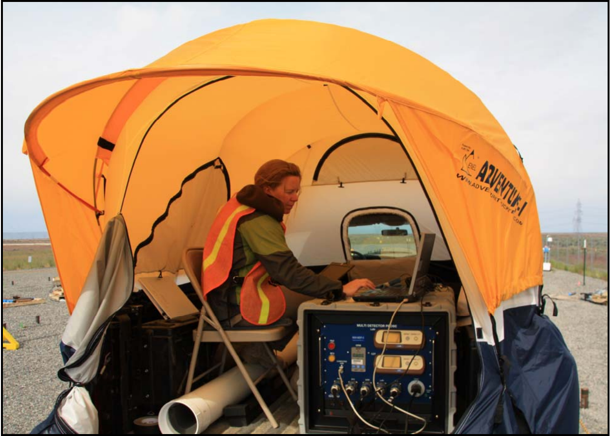
A North Wind employee takes readings during nonintrusive characterization of the vertical pipe units at the 618-11 Burial Ground. (Photo 8)
