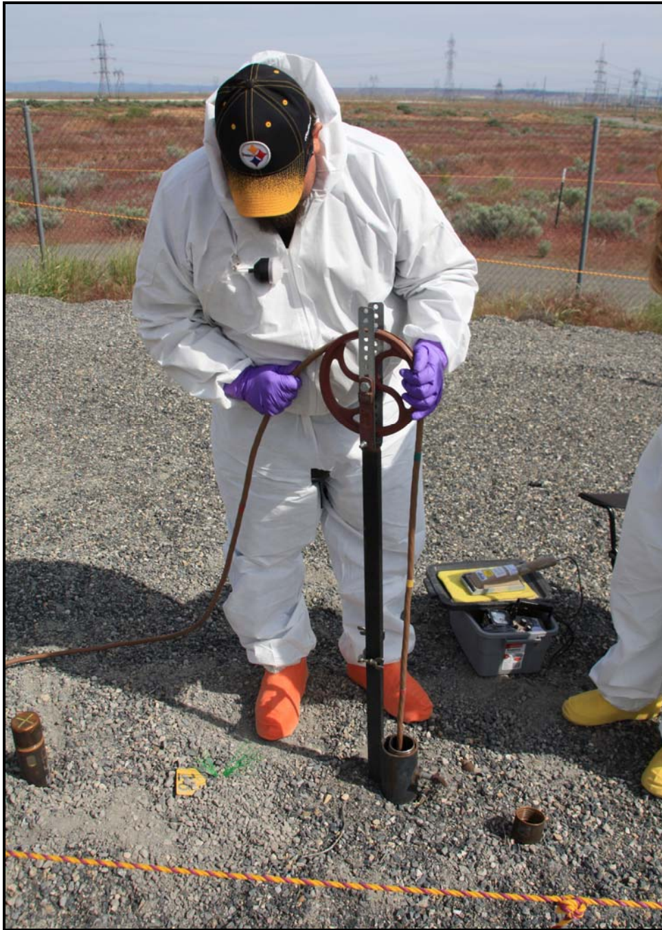
An employee with Washington Closure Hanford subcontractor North Wind Inc. lowers a multi-detector probe into a cone penetrometer to characterize a vertical pipe unit at the 618-11 Burial Ground. (Photo 6)
