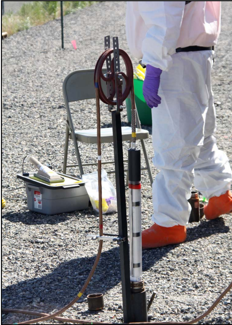
A multi-detector probe is a gamma-logging instrument used to determine the location of the radioactive materials within a vertical pipe unit. (Photo 8)
