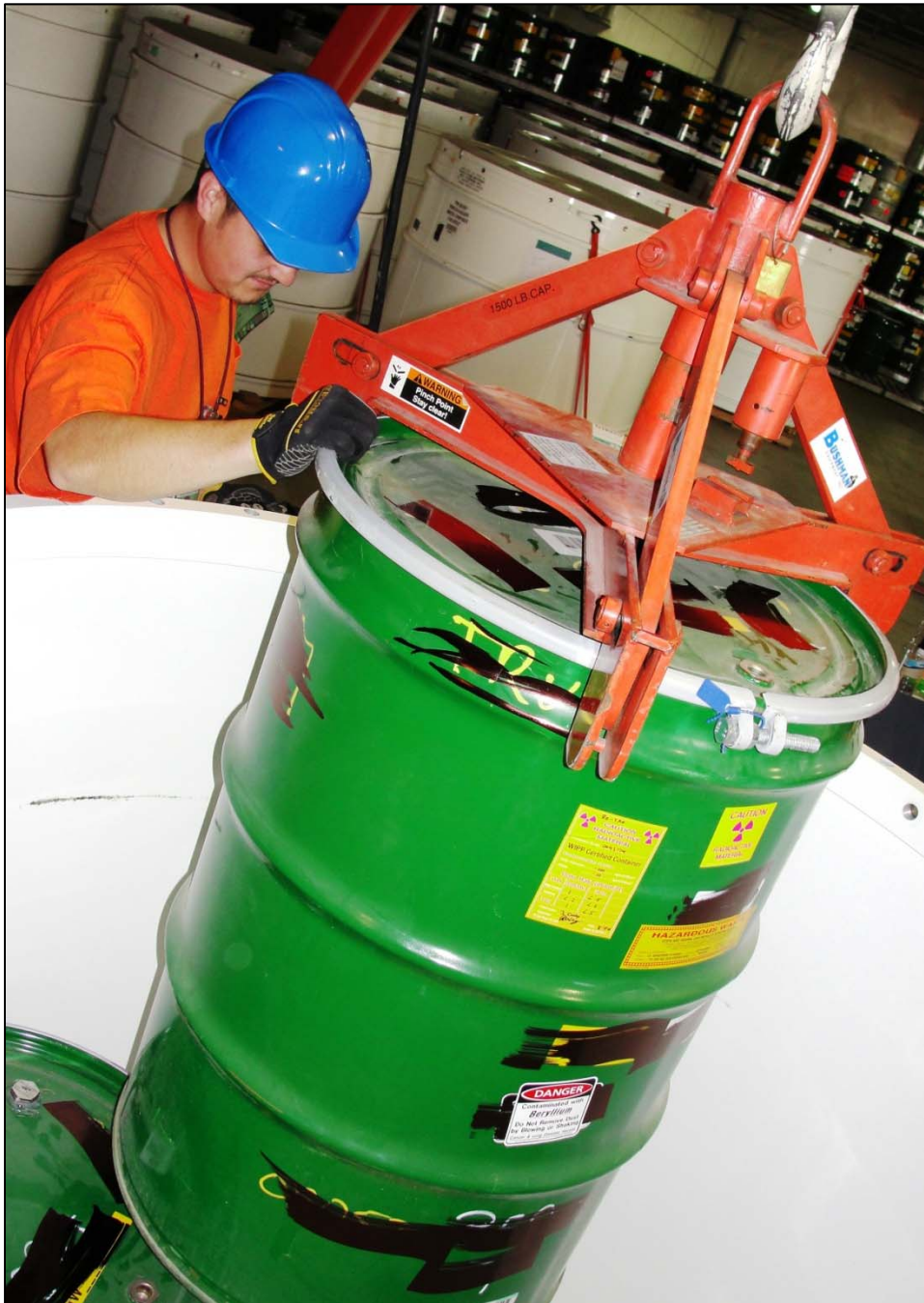
A worker loads a drum into a ten-drum over-pack container in preparation for the TRUPACT-II shipment leaving the Waste Receiving and Processing Facility.
