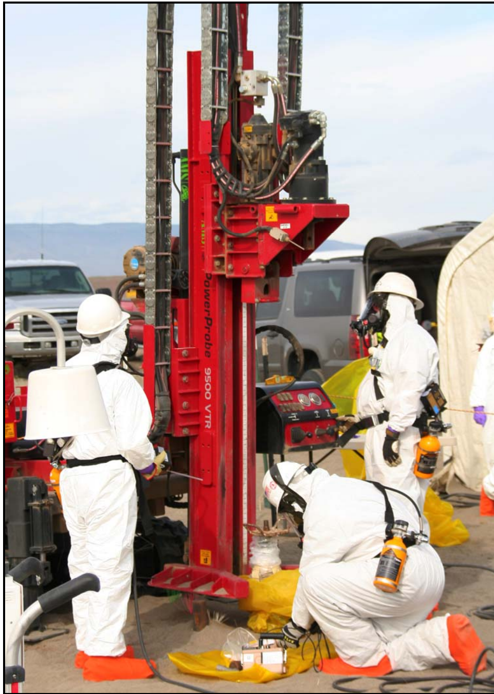
The project team drives a cone penetrometer to obtain a soil sample at the 618-10 Burial Ground. The cone penetrometer is driven about 2 feet below the vertical pipe unit.
