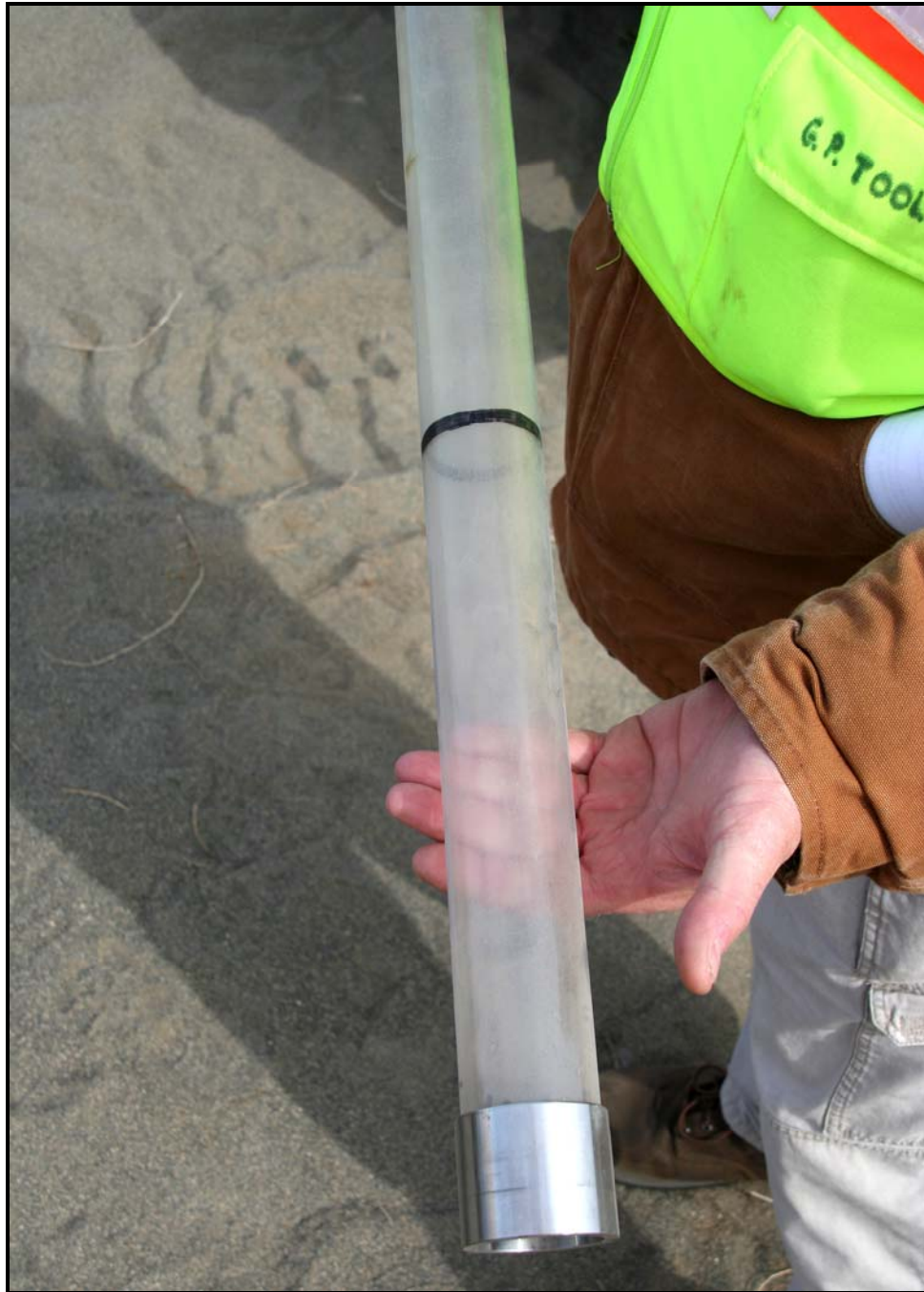
A sampling tube is used to collect soil during nonintrusive characterization activities at the 618-10 Burial Ground.
