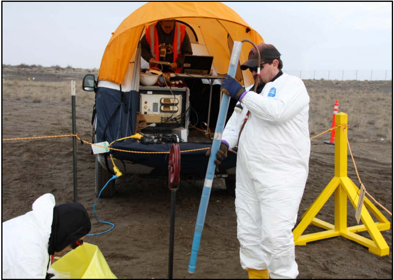
North Wind Inc. employee prepares a multi-detector probe for use at the 618-10 Burial Ground.
