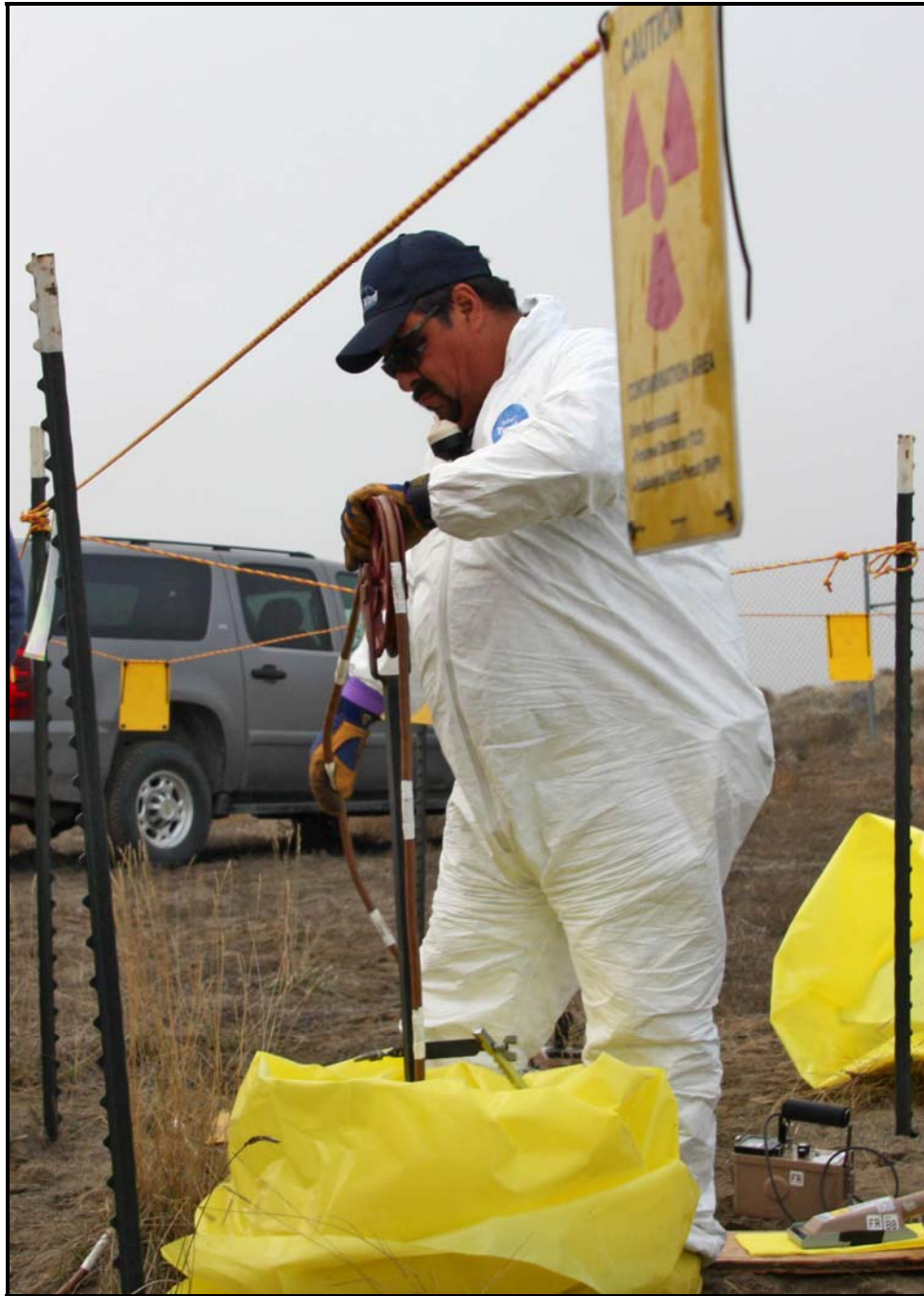
A North Wind Inc. employee retrieves a multi-detector probe during radiological characterization activities at the 618-10 Burial Ground.
