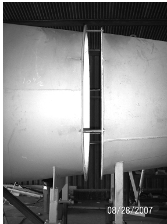
Figure 6.7. Gap in shock tube used to simulate negative phase pressures (PDC 2007).
