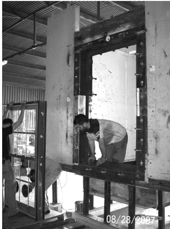
Figure 6.8. Shock tube side of the reaction structure (PDC 2007).
