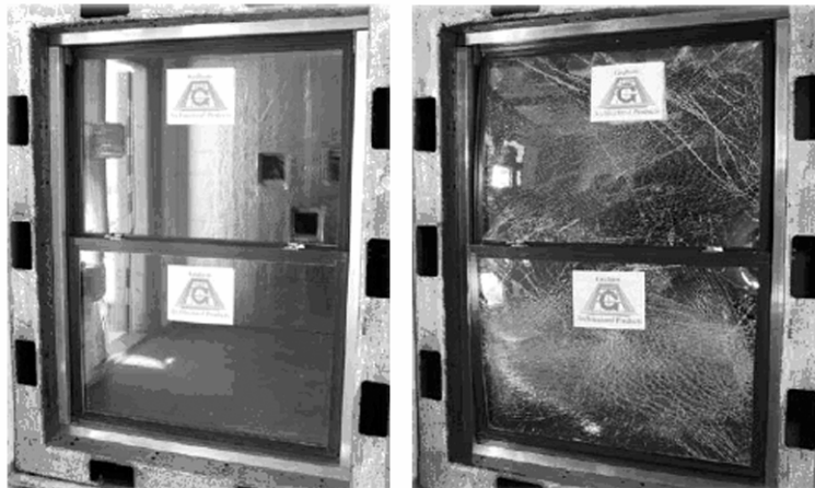
Figure 2.4. Pre- and post-blast test views of laminated glazing. Note that fractured glazing remains in its frame (Graham Architectural Products website).
