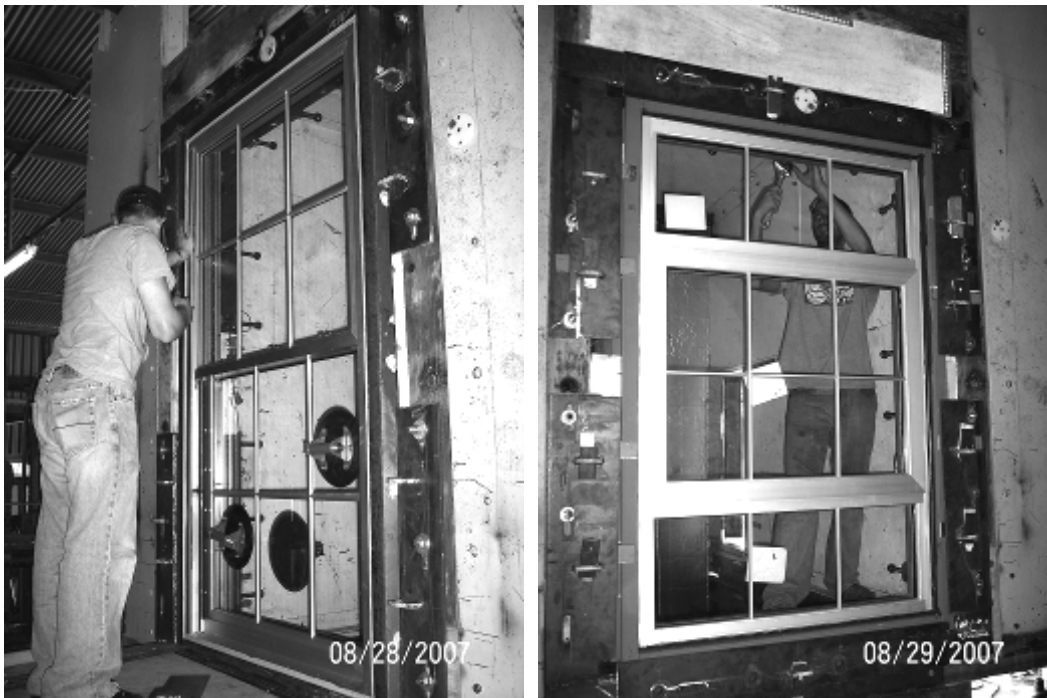
Figure 6.9. Hung window specimen (left) and factory window specimen (right) installed in the reaction structure (PDC 2007).
