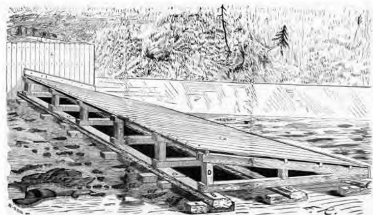
Hollow Frame Dam
