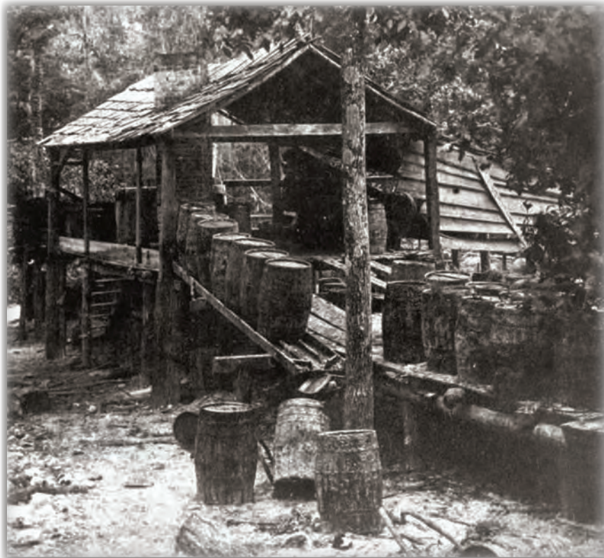
Emptied Barrels Being Drained of Crude Turpentine Residue. Note the draining channel on the ramp with spout and collection barrel. Unknown Location and Date (Florida State Library).
