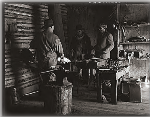
Detail of a Blacksmith Shop Showing the Anvil Base and Stand Forge with Blower. New Mexico, 1944 (Library of Congress).
