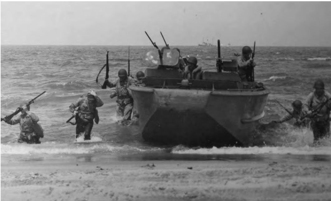
Figure 221. A landing craft, personnel (LCP) with full infantry load (38 men) in training operations on the Atlantic coast with Mark 21-30 caliber machine guns, 21 August 1943 (NARA College Park, RG 80-G, box 393, photo 85163).
