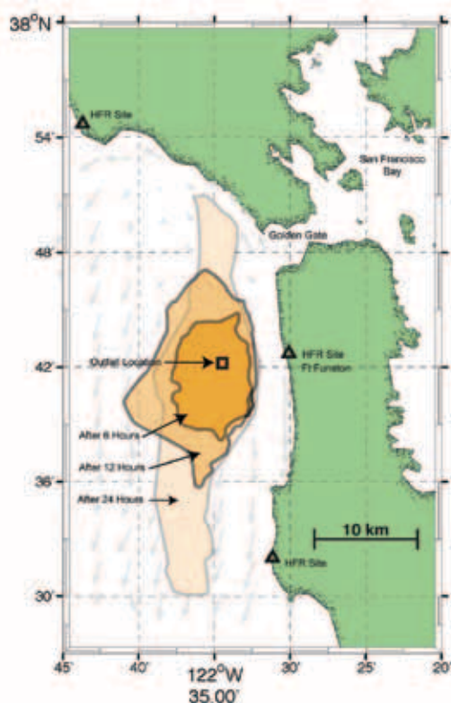
Figure 6: Trajectory forecasts during the Ocean Beach Outfall near San Francisco derived from near-real-time HFR data.
