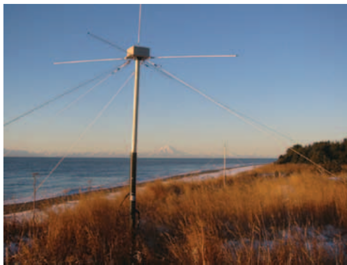
Photo 3: Coastal Ocean Dynamics Applications Radar (CODAR) Receive Antenna (foreground) with Transmit Antenna in background. Cook Inlet, Alaska.
