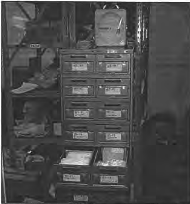
Figure 101. A metal storage unit with drawers houses small artifacts with paper and plastic envelopes as primary containers. A hygromograph on the unit monitors both temperature and relative humidity.
