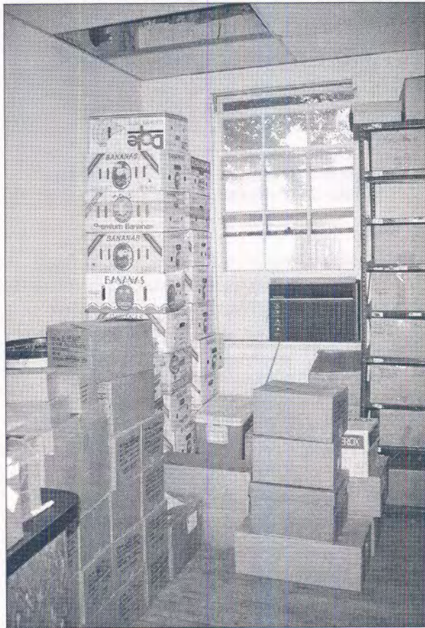
Figure 13. Vertical stacking of boxes causes compression damage, and proximity to windows poses a security risk at NCOSA.
