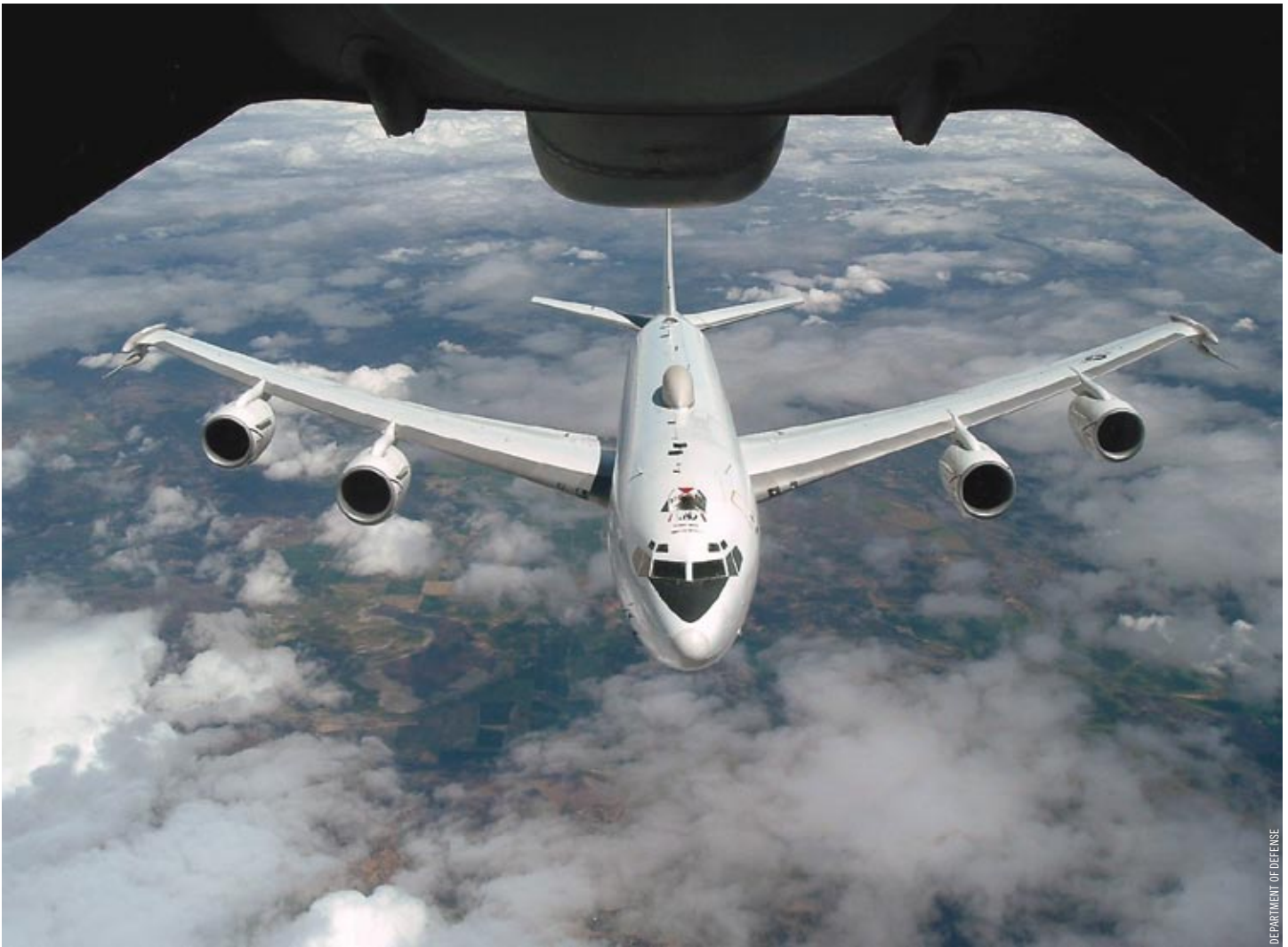
(above) A “Looking Glass” E-6B Mercury aircraft approaches an Air Force KC-10A Extender for aerial refueling. The E-6B can be refueled repeatedly to keep it airborne as long as needed. (page 22) A Strategic Air Command airborne command and control crew turns the missile launch keys aboard the EC-135 “Looking Glass” that preceded today’s E-6B.
