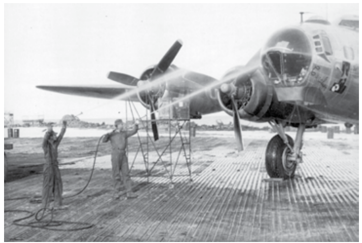
(above) Crew members decontaminate a B-17G Flying Fortress after a nuclear weapon test. Vehicles, planes, and even some of the target ships used in multiple tests had to be scrubbed down or hosed off after each test, although underwater and high altitude bursts usually had less or little ionizing radiation compared to tests on land. (left, top) Operation HARDTACK I, June 8, 1958. The ship in the foreground is the SS Michael Moran , a mothballed Liberty ship used as a target in two underwater nuclear weapons tests, Shot WAHOO and Shot UMBRELLA (pictured here), conducted near the Enewetak Atoll in the Pacific Proving Grounds. (left, bottom) Operation BUSTER-JANGLE, Nov. 4, 1951. Exercises Desert Rock I, II and III were conducted during this test series (Shot DOG pictured here); thousands of troops from all four branches of the military participated in observer programs, tactical maneuvers and damage effects tests.
