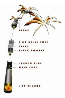
**Figure 3-1: Display Firework Schematic** (from <u>www.pbs.org/wgbh/nova/fireworks/anat\_flash.html</u>)
