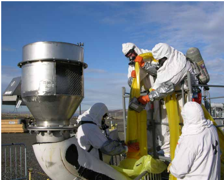
Workers deploy a sampler system in a single-shell tank to obtain previously inaccessible waste samples.
