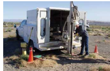
A geoprobe is used to collect soil samples to test for contamination.
