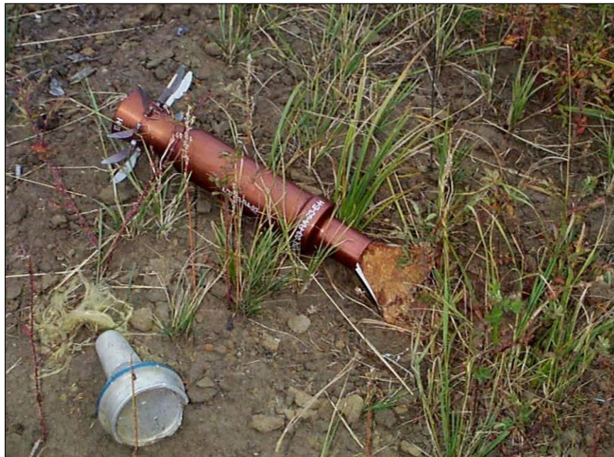
Figure 11. Ruptured LAW rocket at CFB-Valcartier, amber solid is octol, the color results from photolysis of the TNT component.
