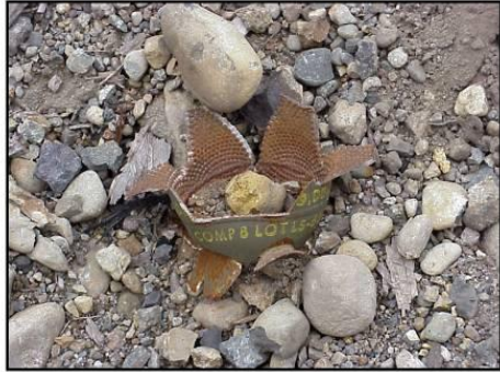
Figure 8. Hand grenades that did not completely detonate.
