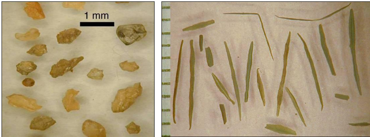
Figure 24. Examples of energetic material particles: TNT particles (<1 mm, fraction) from a blow-in-place detonation (left), 105-mm howitzer propellant fibers from a collection tray 3 m from muzzle (right, 1-mm scale).
