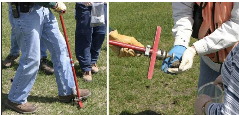
Figure 27. Coring tool designed specifically for collecting cohesive multi-increment soil samples.
