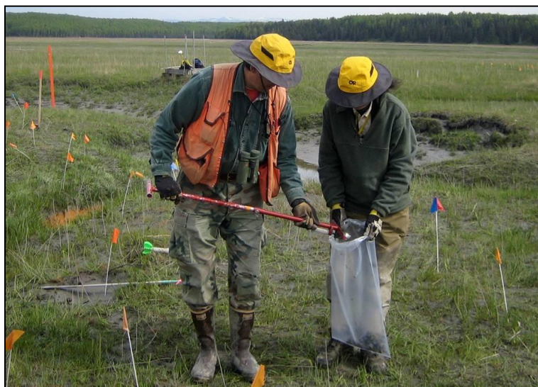
Figure C-8. Photo of a two-person team collecting a multi-increment sample.
