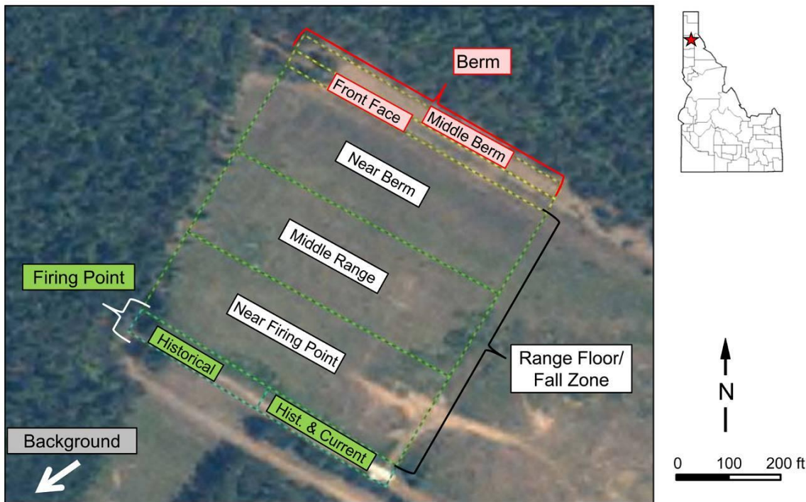
Figure A5-1. Air photograph of the Farragut firing range with overlays showing the boundaries of the sampling units. Inset shows the general location of Farragut. (after Techlaw 2010).
