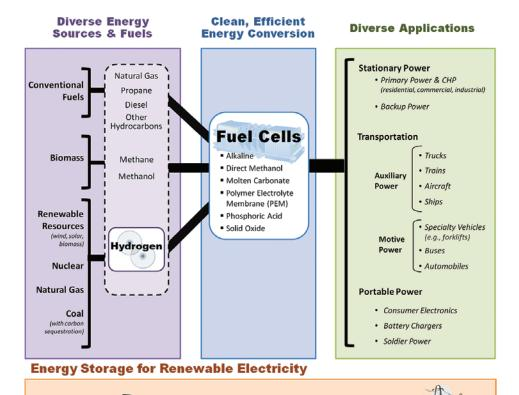
Hydrogen and fuel cells can be used in all sectors of the economy, providing a highly efficient means for producing electricity from a number of energy sources (including natural gas and abundant, renewable domestic resources). Hydrogen can also be used for energy storage and delivery, offering potential benefits for intermittent renewable power generation. Illustration by Fuel Cell Technologies Program, EERE
