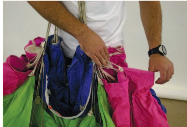
Figure 4-8. Clear the stabilizers on each side.
