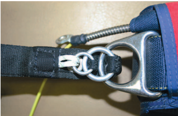
Figure 4-39. 3-ring loop over top ring.
