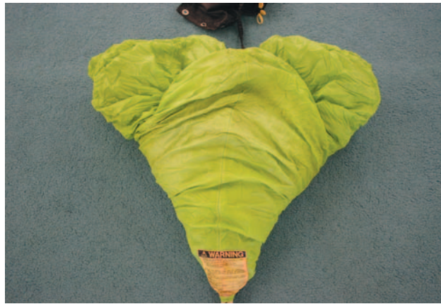
Figure 4-20. Triangular shape on the floor. Make sure the slider is securely wrapped in the tail.
