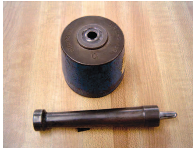
Figure 6-52. Size “O” rolled rim spur grommet handset.
