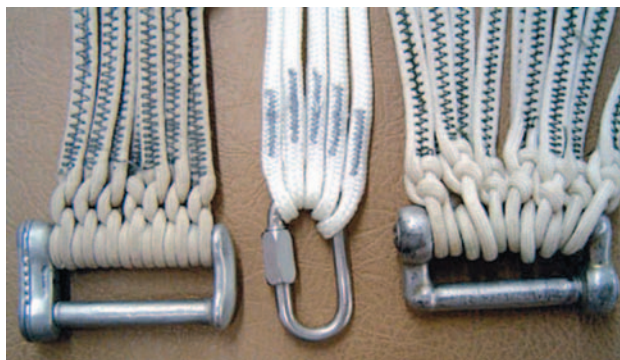
Figure 5-14. Three types of connector links.
