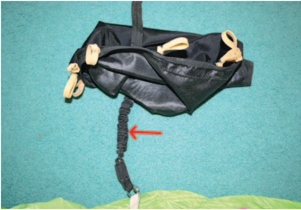
Figure 4-22. Check the collapsed bridled.
