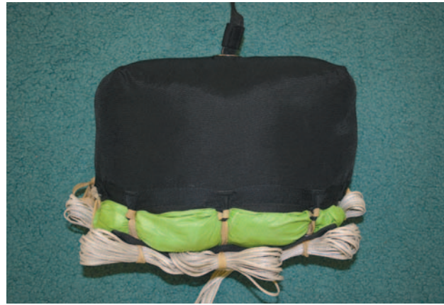
Figure 4-32. Stow the remainder of the lines on the side bag stows.
