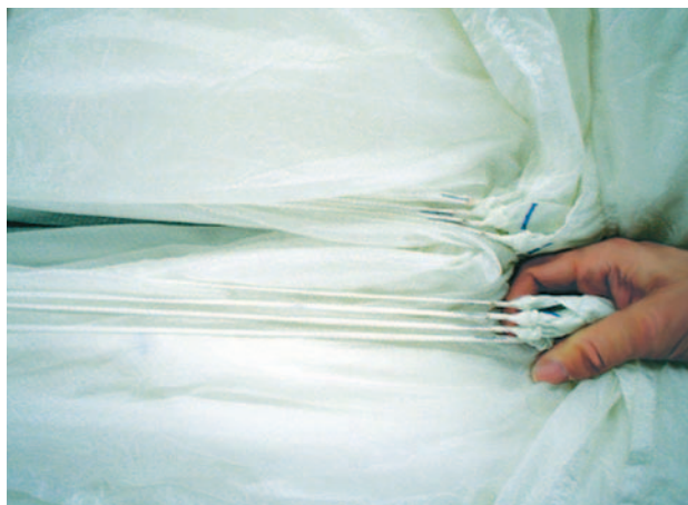
Figure 5-88. Lines are taut in the center.
