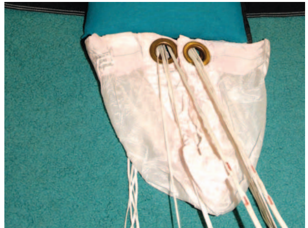
Figure 5-72. Pull slider down.
