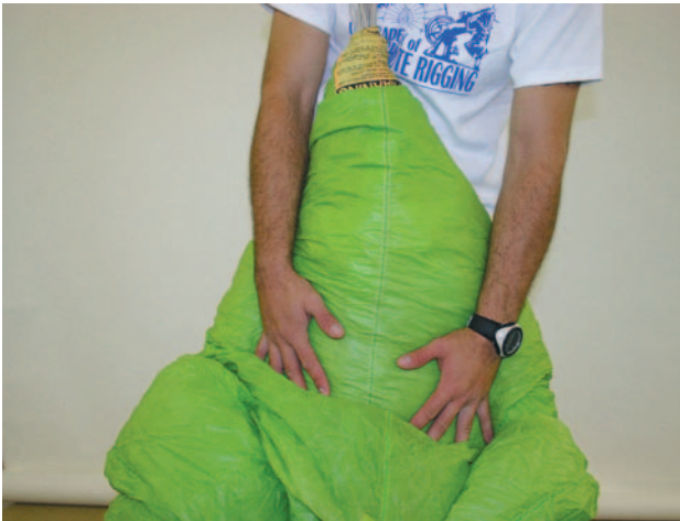
Figure 4-17. Smooth the air out of the rolled canopy.
