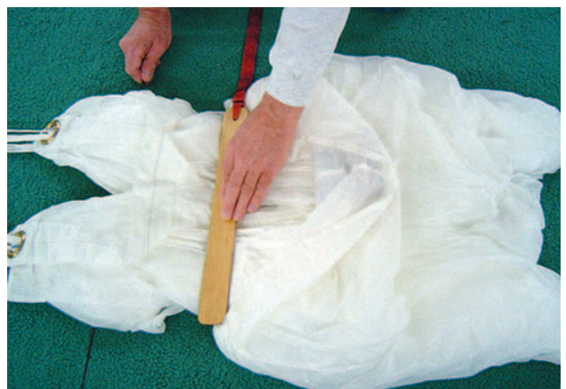
Figure 5-91. Packing paddle at 1/3rd location.
