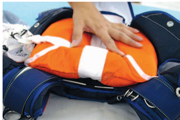
Figure 5-106. Fold the yoke over the bridle.
