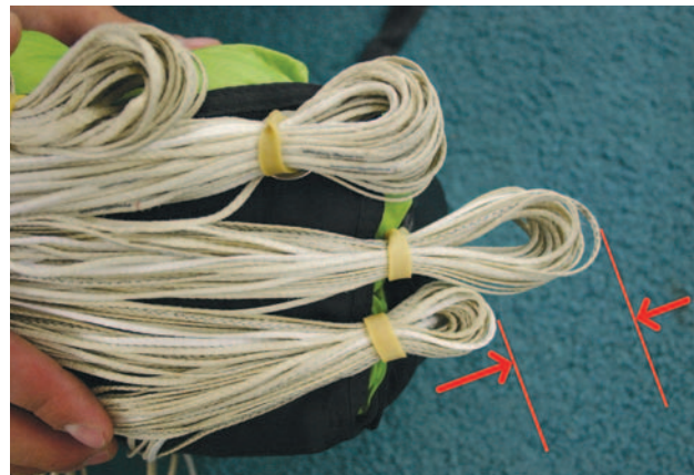
Figure 4-35. Line stow length comparison.
