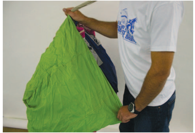
Figure 4-13. Grasp the center of the tail seam with the same hand that holds the lines. With the other hand, pull the tail seam downward. Repeat for the other side.
