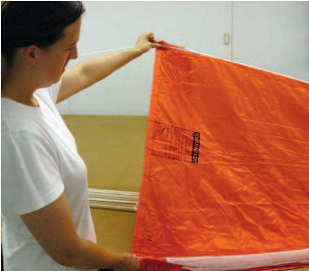
Figure 5-11. Round canopy gore inspection.
