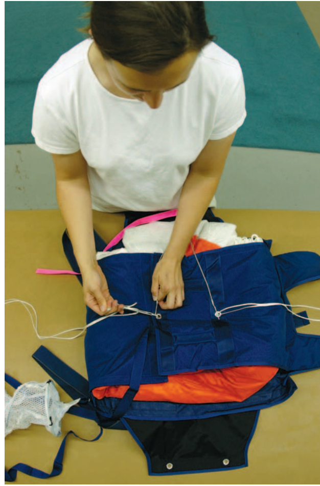
Figure 5-60. Closing bottom flap.
