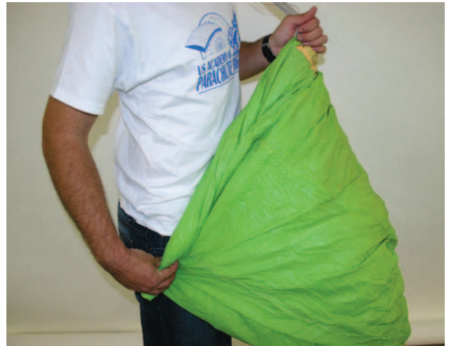
Figure 4-15. Roll both seams together tightly starting at the bottom.
