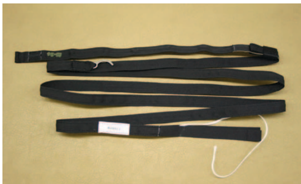
Figure 2-35. Kill-line collapsible bridle.
