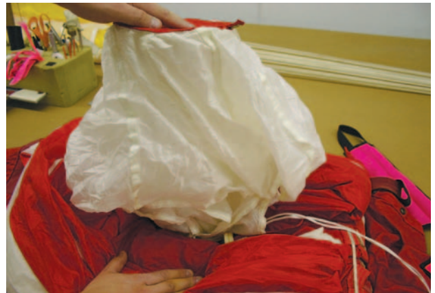
Figure 4-49. Type 1 deployment in a pilot emergency rig.
