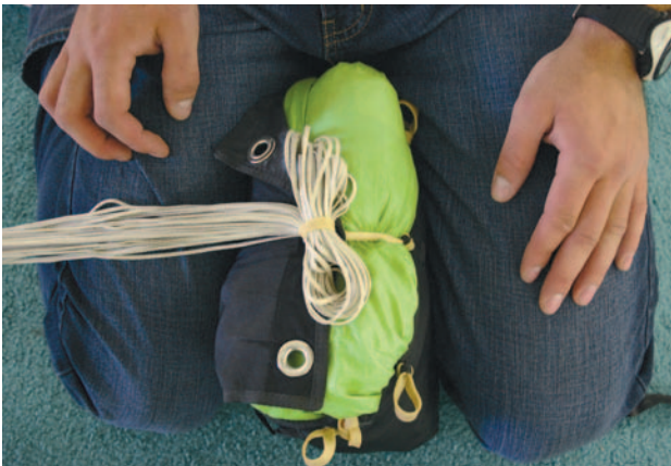
Figure 4-30. Secure the center locking stow with the line group.
