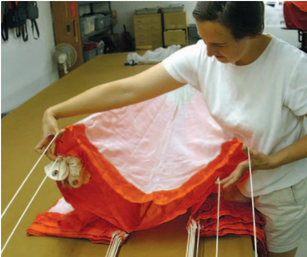
Figure 5-8. Round canopy—four-line check at canopy.
