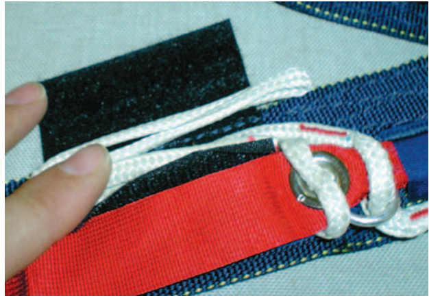
Figure 5-84. Set the deployment brakes.
