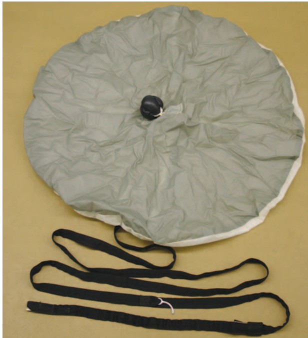
Figure 2-40. TOP bridle/pin configuration.
