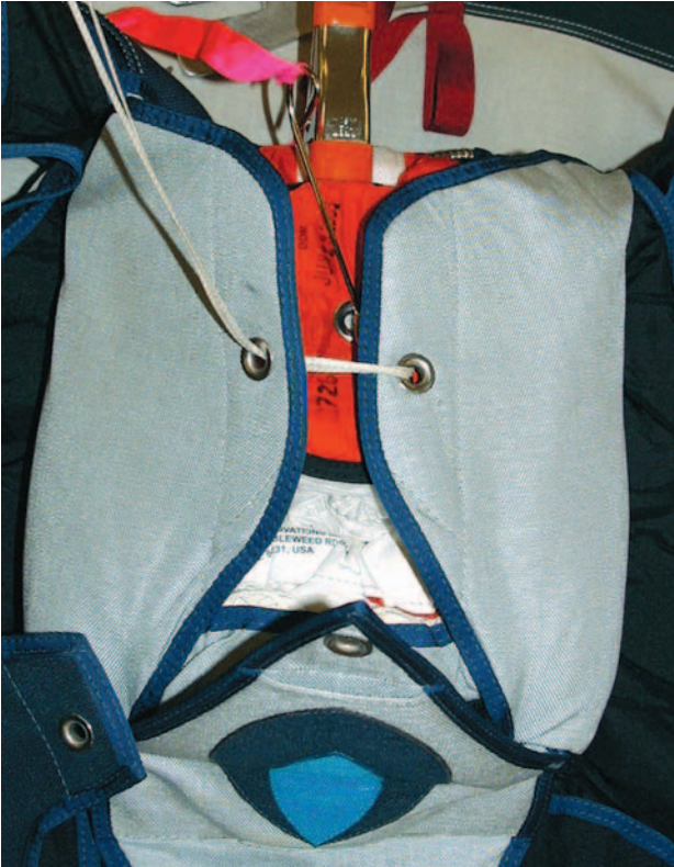
Figure 5-111. Close right and left flaps simultaneously.
