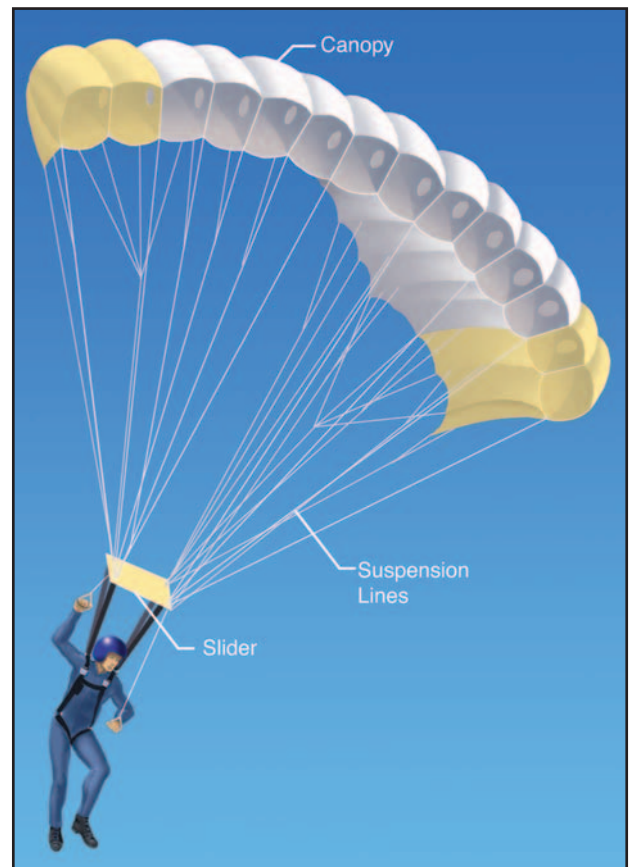
Figure 2-1. Component parts of a main parachute assembly.
