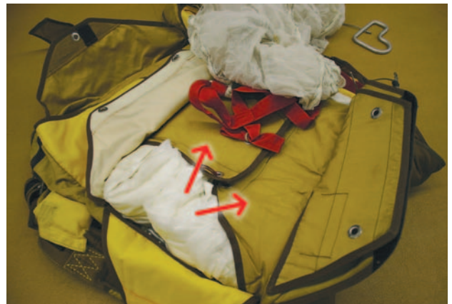
Figure 4-50. Type 1 deployment in a sport piggyback.
