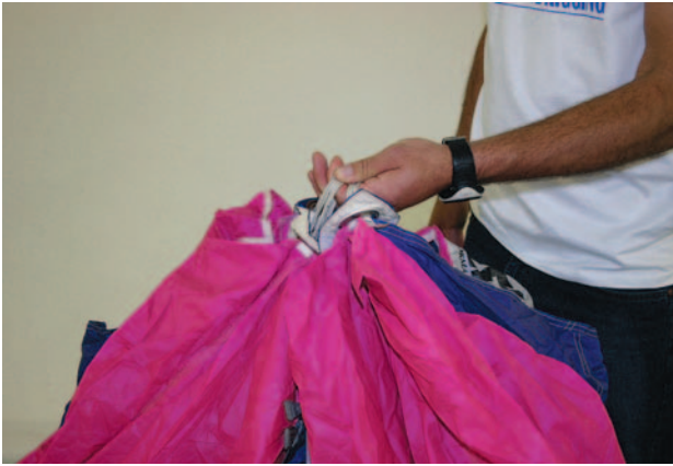
Figure 4-5. Transfer all the lines to one hand.
