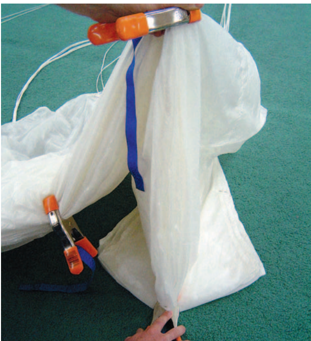
Figure 5-78. Hold "B" clamp vertically over "A" clamp.
