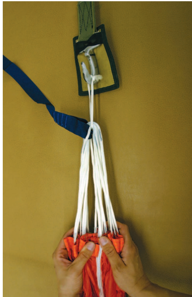
Figure 5-34. Straightening the canopy apex.
