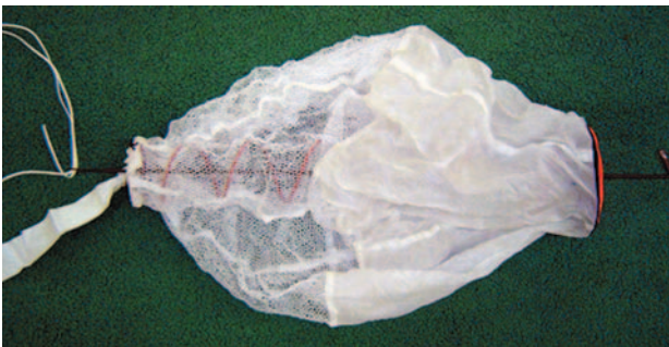
Figure 5-108. Gun rod through the pilot chute.
