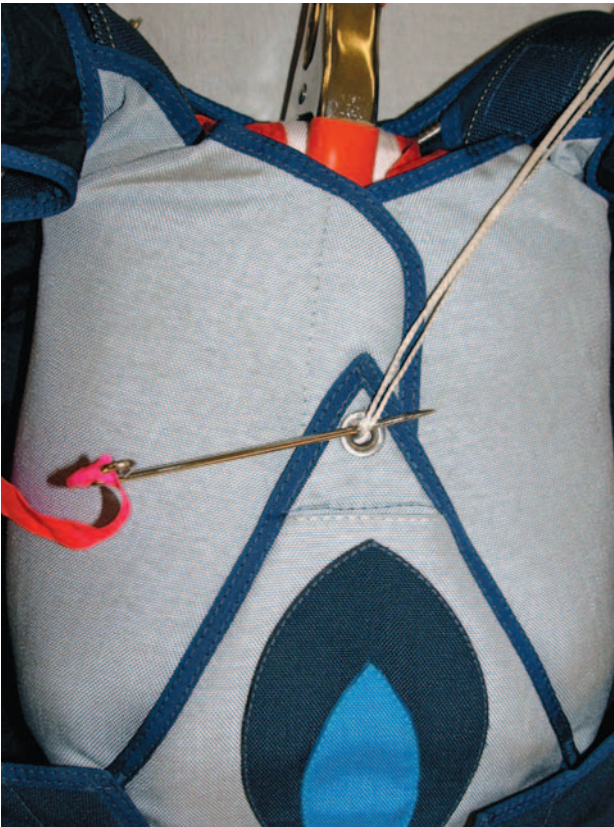
Figure 5-112. Close #3 bottom flap.
