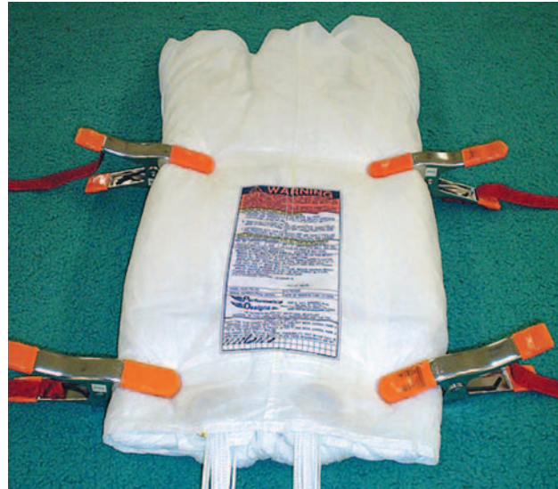
Figure 5-94. Finish wrapping tail, four clamps.
