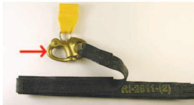
Figure 2-52. Snap shackle on RSL lanyard.
