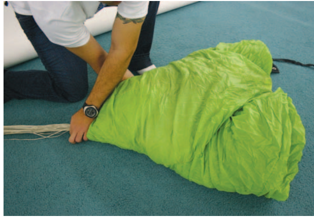
Figure 4-19. Keeping the lines taut, lay the canopy bundle on the floor.
