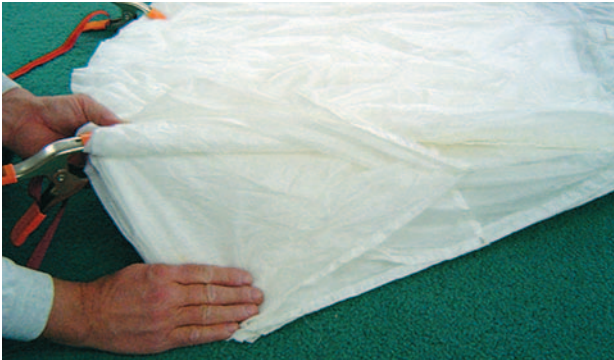
Figure 5-76. Fold half under "A" lines.
