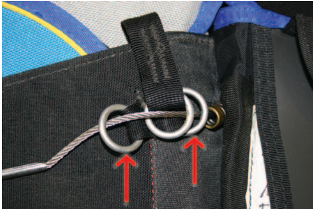
Figure 2-53. Double ring container installation.
