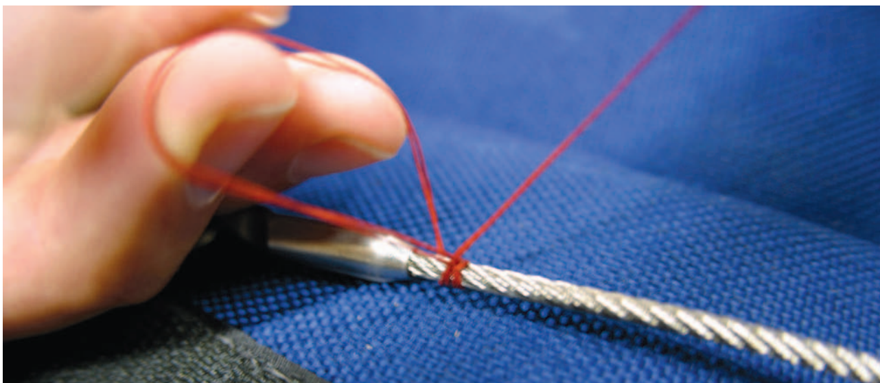
Figure 5-65. Lark’s head the thread on the cable.
