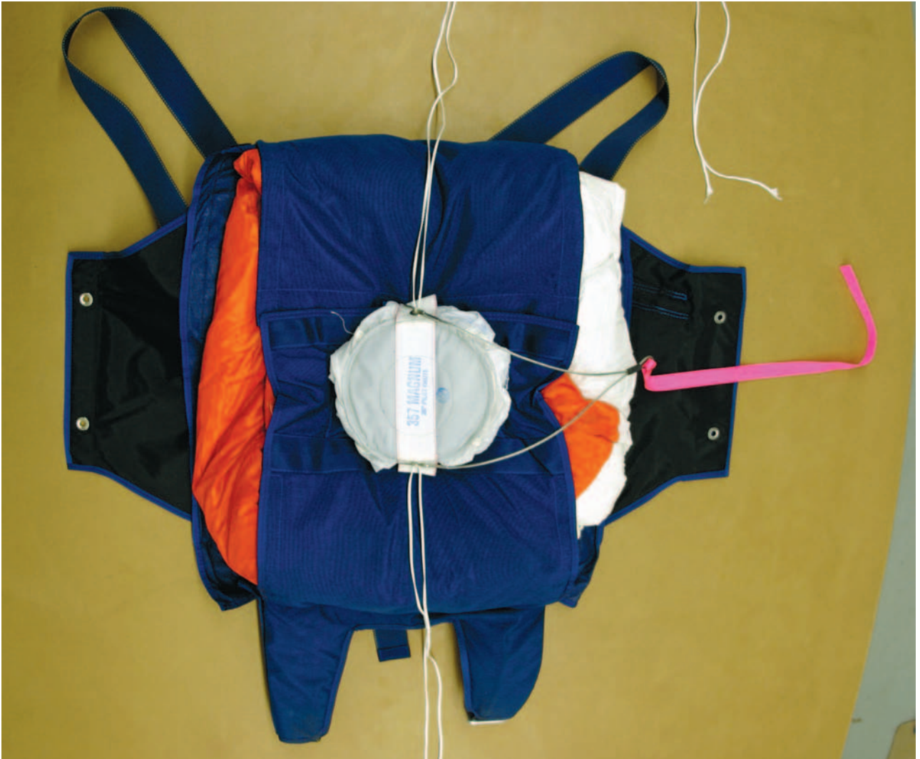
Figure 5-62. Pilot chute seated in position.
