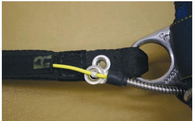
Figure 4-42. 3-ring cable thru loop.
