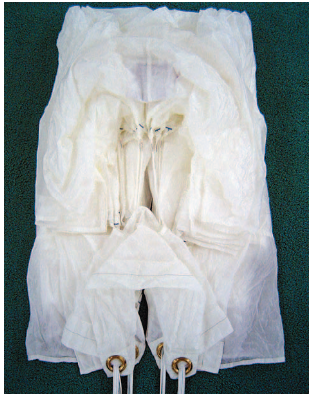
Figure 5-89. Fold tail back for wind channel.
