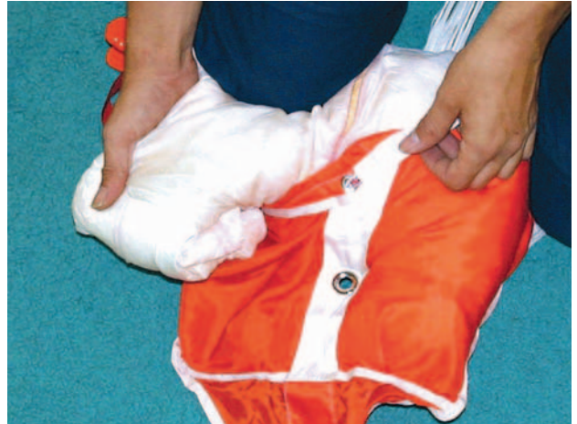
Figure 5-100. Fold molar ends under.
