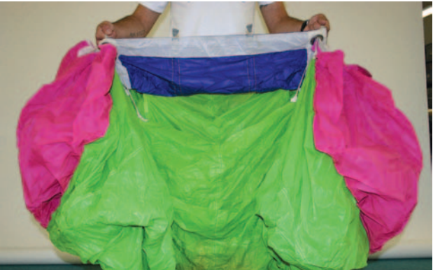
Figure 4-3. Run your hands up the lines pushing the slider ahead of them. Spread the line groups and shake out canopy.
