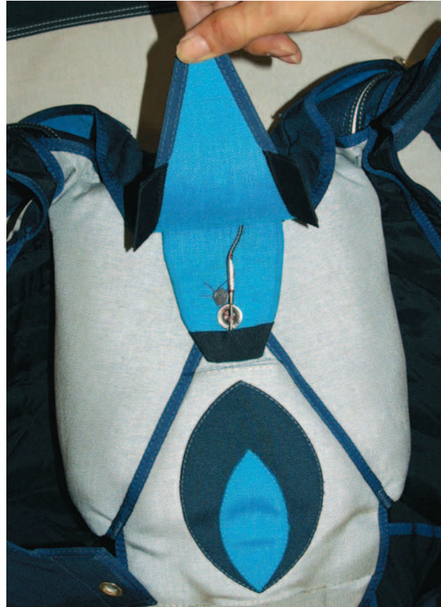
Figure 5-113. Close flap #4 and insert ripcord pin.
