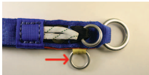
Figure 2-51. Main riser RSL ring attachment.
