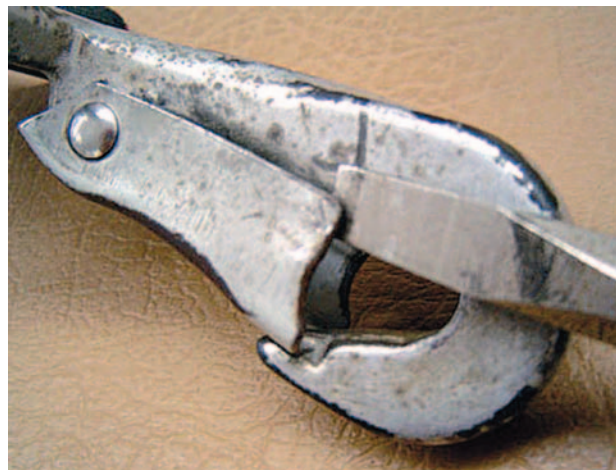
Figure 5-16. B-12 snap gate repair.
