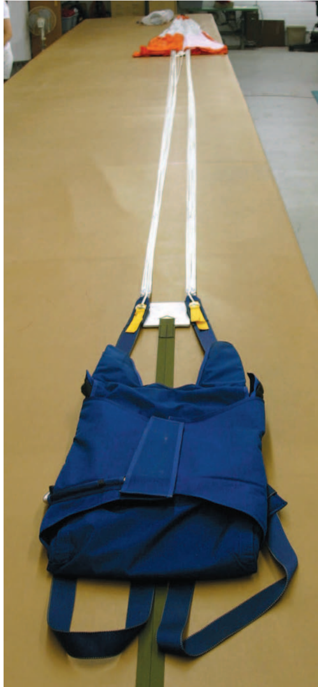
Figure 5-4. Round canopy pilot emergency parachute assembly.
