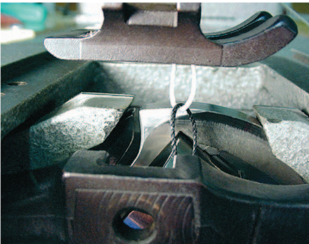
Figure 6-70. Fifth in sequence in forming a stitch.
