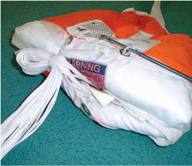
Figure 5-102. Close bag and secure locking stows.
