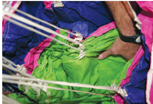
Figure 4-10. Separate and clear material between line groups.
