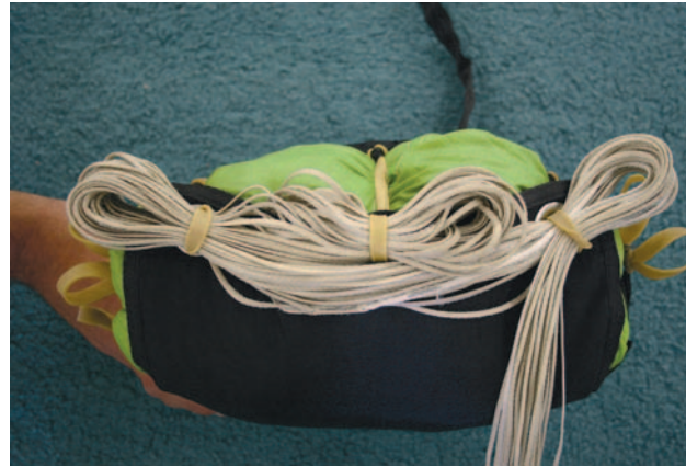
Figure 4-31. Secure the remainder of the mouth locking stows.
