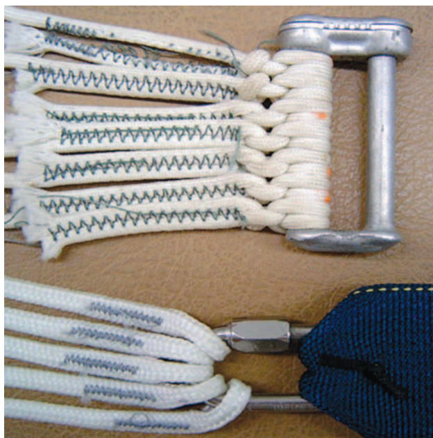
Figure 5-13. Connector link line attachment methods.
