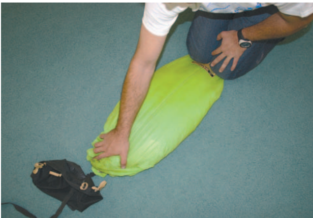
Figure 4-23. Dress the canopy bundle slightly wider than the deployment bag.
