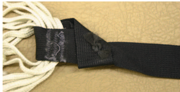
Figure 2-32. Hand tack floating bridle loop.
