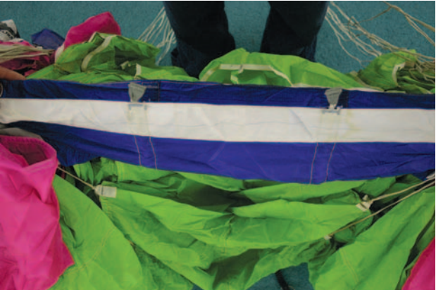
Figure 4-4. Make sure the canopy is orientated with the nose to rear and tail to front. This view is shown from the top of the canopy looking down and towards the packer.
