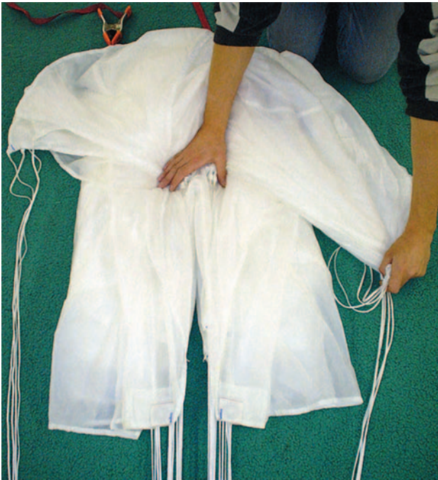
Figure 5-83. Pull down the trailing edge.
