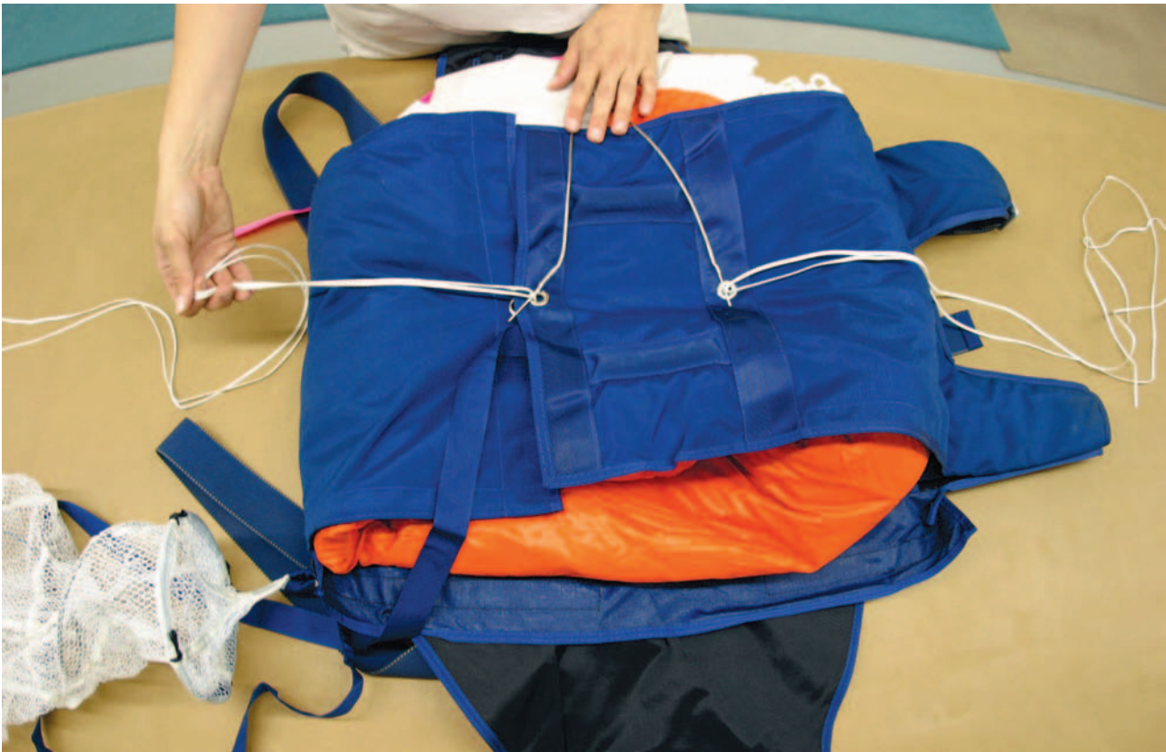
Figure 5-61. Upper temp pin seated.
