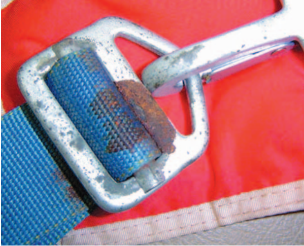
Figure 5-17. Rusty leg snap hardware.
