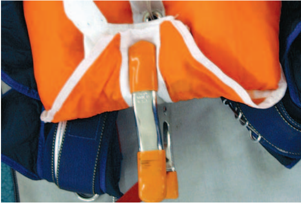
Figure 5-107. Secure yoke/bridle with clamp.
