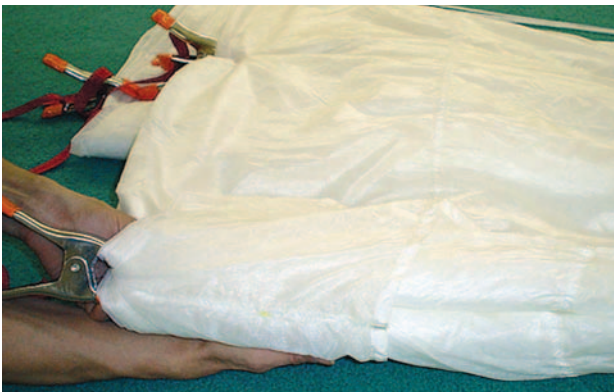
Figure 5-77. Smooth panels under "A" lines.
