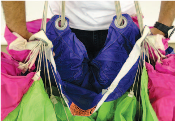
Figure 4-11. Square the slider between the line groups.
