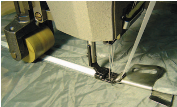
Figure 6-82. Tape feeder and French seam folder.
