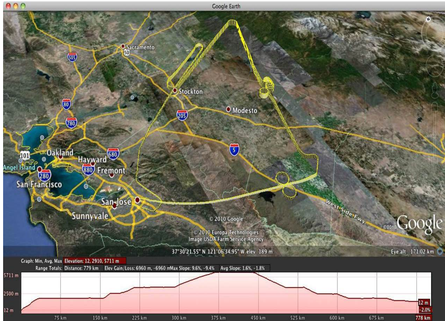
Figure 1. Flight track of G-1 4STAR test flight on September 28, 2010, out of Moffett Field, California. The yellow curtain plot shows the various flight maneuvers executed during this first test flight. The bottom strip chart indicates the flight altitude profile from take-off to landing.
