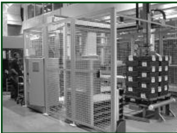
The Bureau's new robotic currency palletizer eliminates the need to physically lift and stack cash packs.
