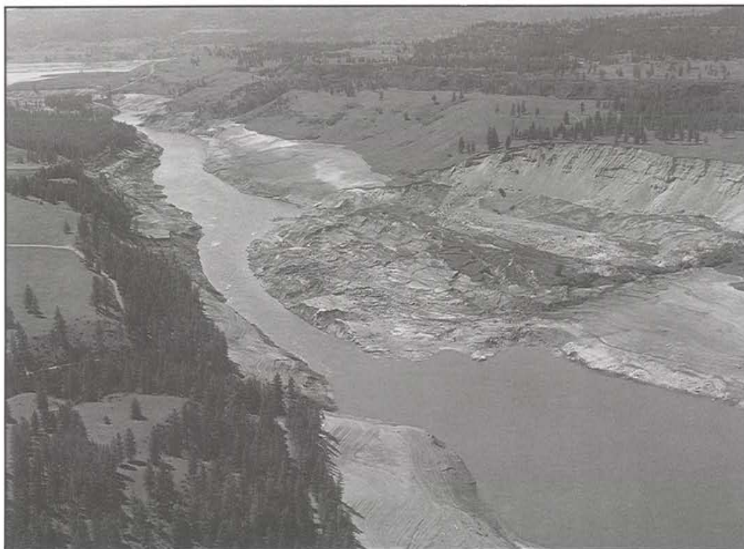
At Grand Coulee, the river bank is prone to collapse into the river. The Bureau of Reclamation has set a maximum draft limit that allows the bank to drain, reducing the possibility of sloughing.
