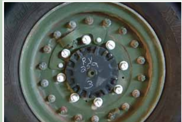
Thin Dense Plated Aluminum coated bolts are installed on Stryker wheel assemblies. After 2.5 years of service in Hawaii, these unpainted bolts, which were exposed to a Tropical Environment, show no sign of corrosion degradation.
