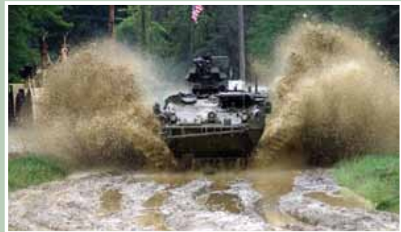
A Stryker in theatre fording a small body of water. These types of environments require a robust corrosion resistant metal/surface finish and Chemical Agent Resistant Coating paint topcoat system. The HazMat free Stryker utilizes recent innovative solutions in surface finishing that meet both corrosion resistance and HazMat elimination requirements.
