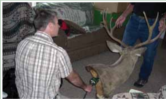
Using a device known as a HAPSITE, Hill AFB workers identify this stuffed deer head as the source of volatile organic compound (VOC) vapors in a home. If the Air Force can trace VOC vapors to an inside source, it saves them thousands of dollars that would have otherwise been spent installing and maintaining a vapor mitigation system.
