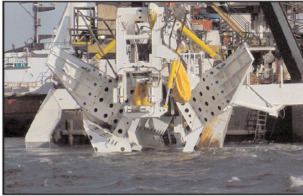
Figure 4-4 A Typical Pipeline Burial Plow (courtesy of Horizon Offshore)
