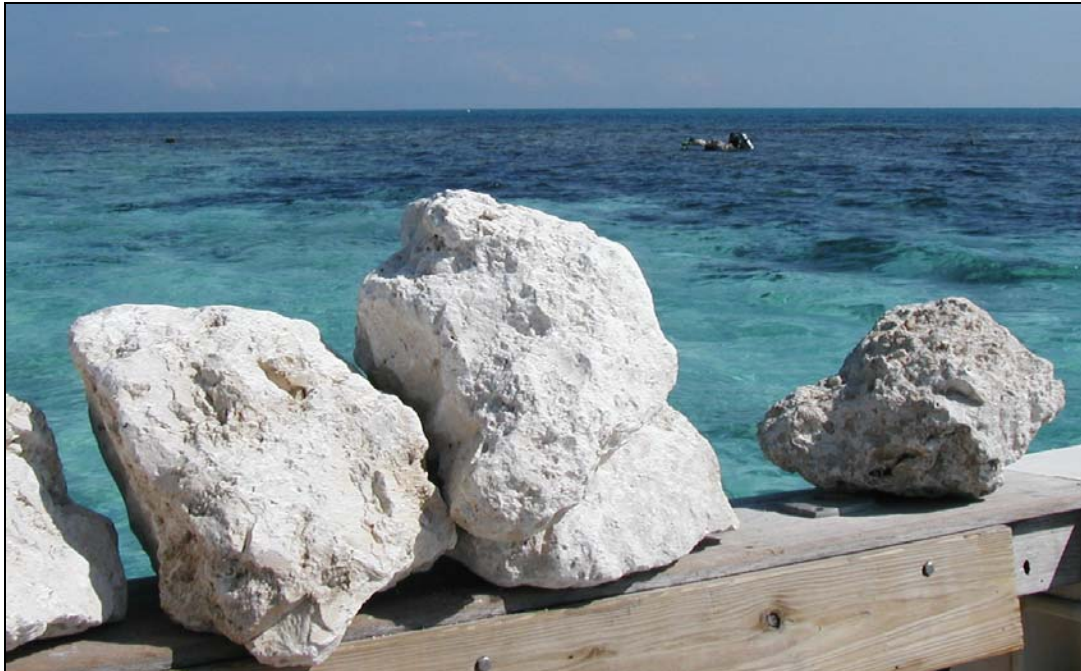
Figure 11 Limestone Boulders (Size Range of 1 to 1.5 feet [0.3 to 0.5 meters]) Representative of Those Suggested for Mitigation to be Used to Mimic the Low-relief Structure of the Natural Hard Bottom Habitat
