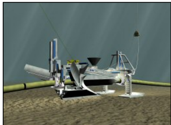
Figure 5 Monitoring and Adjustment of Ditch Being Cut
