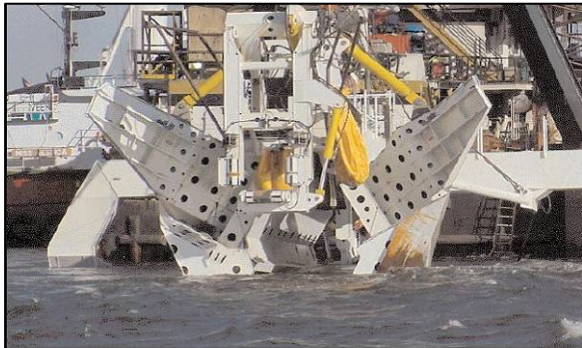
Figure 2 A Typical Pipeline Burial Plow (Courtesy of Horizon Offshore)
