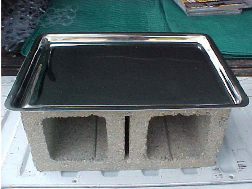
Figure B2. Example of a Sediment Accumulator Plate (Source: Broward County Undated)
